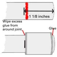
■ 4. Run a line of glue around the motor mount tube where the red line indicates. Slide on the shroud ring (C) and seat it in the glue, making sure it is flush against the bottom ring of the adapter. Make a fillet of glue around the joint.
