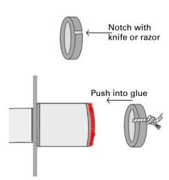
☐ 6. Feed the Kevlar cord through the motor tube and out the bottom. Apply glue to the inside of the main airframe (I). Insert the motor mount assembly until the shroud ring is flush against the bottom of the tube.
