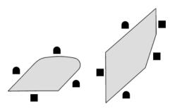
□ 22. Lay a pod tube assembly on the pod fin jig so the mark is just a little below the bottom edge of the jig. Lay the outer fin flat on the jig and line the trailing edge up with the mark. Tack the outer fin in place with CA glue. Do the same for the inner fin. Repeat to make three fin/pod units.
