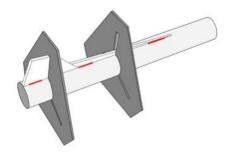
☐ 15. Apply white glue fillets at the fin/airframe joint on both sides of all three fins.
