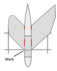
☐ 23. When all three pod units have fins tacked in place, apply fillets of white glue to all fin/pod joints.
