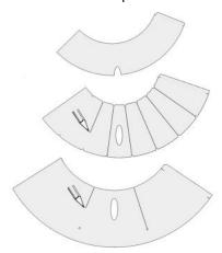
**8.** Gently curl the shrouds over the edge of a table or a ruler. Take care to not bend or tear the shrouds, especially near the launch lug holes.
