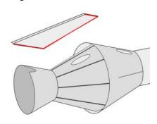
□ 25. Insert the launch lug (J) into the shroud assembly until it is even with the bottom of the nozzle shroud. Glue into place as shown. After the glue sets, cut the launch lug to the angle of the top shroud with a sharp knife.
