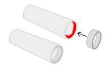
□ 3. Make a mark on the motor mount tube 1 1/8 inches from the end with the motor block. Apply white glue around the motor tube inside of this mark as shown. Take the assembled coupler-adapter ring unit and slide it on until one ring is even with the 1 1/8 inch mark. Apply a fillet of glue around both joints. Wipe away any excess glue and set this assembly aside until the glue is dry.
