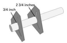
☐ 14. Slide a completed fin into the upper fin alignment jig and tack in place with CA glue where indicated. Attach all three fins the same way. Avoid gluing the fin jigs to the airframe. When all three fins are tacked in place, remove the jigs.
