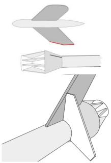
☐ 27. When the glue has dried on the main fins, apply white glue fillets at the fin/airframe joint on both sides of all three fins.
