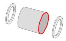
**2.** Glue the motor block (E) into the end of motor tube (D). Smear a line of glue inside the tube, then insert the motor block. Press the tube against the table until the block is even with the end of the tube.
