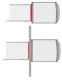
□ 5. Locate the Kevlar anchor (H) Lightly notch the outside of the ring with a hobby knife or razor. Tie the Kevlar cord (Y) in a double knot around the ring so the Kevlar is in the notch. Run a bead of glue around the top of the motor mount. Slide on the notched centering ring with the attached Kevlar and press it gently into the glue. Wipe away any excess glue. Allow time to dry.
