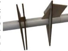
**8.** Glue the upper body tube to the coupler that is attached to the lower body tube. Make sure to feed the shock cord through the tube before sliding the tube onto the coupler. Once you start sliding the tube on the coupler, don't stop until it has seated against the other tube or it will seize and not seat on the coupler fully.
