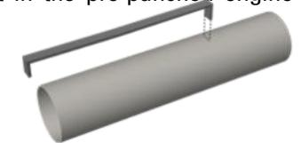
❑ 3. Carefully detach the centering rings (CR-57EH) and slide the ring with the notch over the engine tube. Align the notch over the engine hook and slide it about 1" from the bottom of the engine tube as shown.
