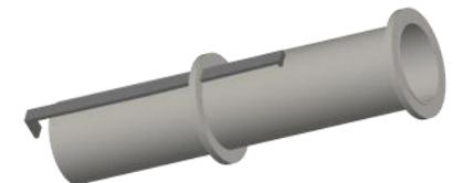
❑ 5. Glue one end of the streamer (SP-110) to the engine tube, centered between the two rings. Some glues will not stick to the plastic material. In this case, you can use masking tape to attach the streamer.
