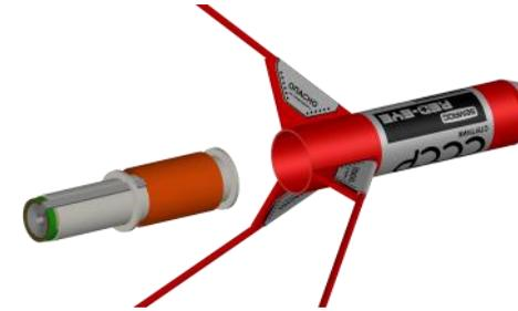
❑ **16.** Refer to the model rocket engine manufacturer’s instructions to complete the engine prepping. Different engines have different igniters.
