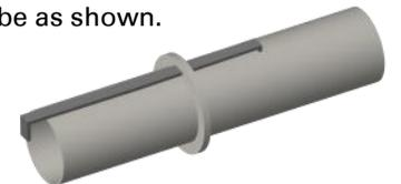
❑ 4. Slide the remaining ring over the top of the engine tube and even with the end of the tube. Apply a bead of glue around both rings at the intersection with the engine tube. Apply a film of glue inside the top of the engine tube. Allow to dry.
