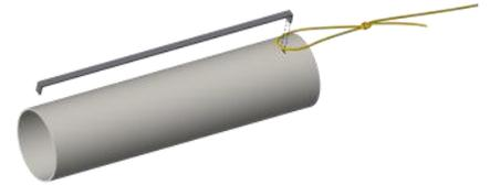
8. Carefully remove the four centering rings from the laser-cut sheet (CR-KV-64). Select the one with four notches and no smaller holes and align the notch over the engine hook. Slide it from the bottom of the engine tube until it is against the end of the engine hook and against the yellow Kevlar® cord.
