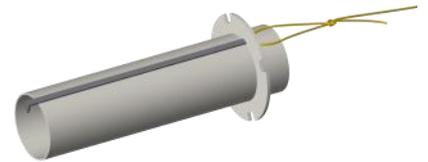
9. Wrap masking tape around the center of the engine tube to hold the engine hook in place and centered along its length. Run a bead of glue over the masking tape and along the engine hook between the tape and the ring. Allow to dry.
