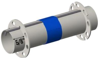
❑ 14. Glue one of the small couplers (HTC-9) in place inside the top of the engine tube and against on top of the engine hook.
