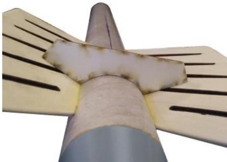
❑ 11. Attach the Launch Lug (I) to the Lower body Tube with the rear most end of the Launch Lug just forward of the leading edges of the fins. Make sure the Launch Lug is parallel with the body tube. After the Launch Lug has had a chance to dry, add glue fillets for extra strength.
