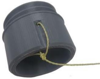
❑ 13. Feed the shock cord back through the coupler so that it comes out the side with the threads. This will get the cord out of the way for when you go to insert the coupler into the body tube.
