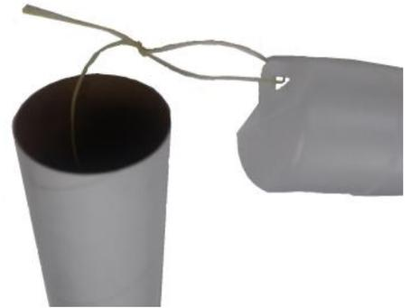
❑ 17. Follow the instructions on the Parachute Package (L) and construct a 15" Parachute. Remove the Nose Cone and attach the Parachute to the Nose Cone where you attached the shock cord. Fold the Parachute and insert it into the body tube and reinstall the nose cone.
