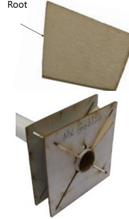
❑ **6.** Using the enclosed fin alignment guides, glue the fins to the body tube. Because of the size of the fins, it is recommended that you use Medium Viscosity Super Glue to initially bond the fins to the body.
