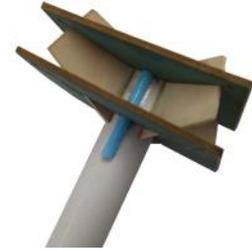
❑ **7.** After you have all four fins attached, glue the plastic Launch Lug to the side of the body tube even with the rear of the body tube. Again use Medium Viscosity Super Glue. After all the fins and the launch lug have dried, add white or wood glue fillets to all glue
