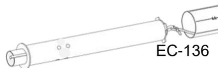
❑ 15. Continue pulling the elastic cord while inserting the top of the engine mount into the main tube. Push it into the main tube until about an inch remains outside the main tube. Run a thick bead of glue inside the main tube and push the engine mount into
