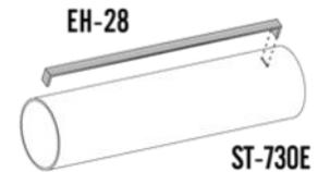
7. Locate the two centering rings. One of the rings (CR-79) is slightly smaller in diameter than the other ring (CR-710). Using the **smaller ring**, slide it over the top (slotted) end of the engine tube until it overlaps the end of the engine hook slightly. **This is important since the wrong combination of rings will not work. If needed, remove one or two layers of paper to make ring fit.**
