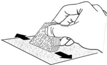
4. Round all the edges except the root edges of each fin. Do not sand the root edge or the tab will not contact the engine tube in a later step.
