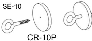
23. Apply a bead of glue just inside the hollow tube coupler (HTC-10). Insert the plywood disc into the coupler and recess it about 1/16". The screw eye should be facing outward. Apply a fillet of glue around both sides of the plywood disk.
