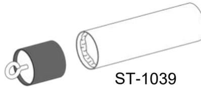
25. Insert the nose cone (BC-1042AC) in the payload tube and check for proper fit. The nose cone should be snug to hold itself in alignment. If it is too loose, add masking tape. If it is too tight, sand the shoulder slightly. If you are not using a payload, the nose cone can be glued in place.
