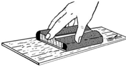
3. Stack all the fins in a group. Line the group up squarely and sand the fins back and forth over some fine sandpaper to get rid of the hold-in tabs as shown below. Do not sand enough to change the shape of the fins.
