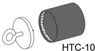
24. Apply a bead of glue inside one end of the payload tube (ST-1039). Insert the tube coupler assembly into the payload tube, leaving 1/2" exposed. Allow to dry.
