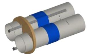
11. Select the other dual engine mount ring and slide it over both engine mounts lining up the engine hook notches with the engine mounts until the second mark at 2-1/4" is just showing. Do not glue yet.
