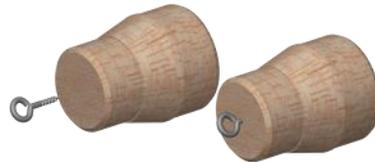
□ 31. Check the balsa reducer (BR-1620S) for fit in the payload tube (ST-2050) and the top of the main body tube. A small amount of sanding may be necessary. Apply a thin bead of glue just inside one end of the payload tube. Insert the balsa reducer until its shoulder is flush with the payload tube. Allow to dry.
