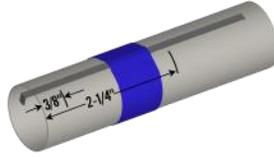
❑ 18. Select the remaining ring with no slot on the outer edge. Align the small notch over the engine hook. Slide it from the bottom of the engine tube until the mark at 3/8" is just showing. Do not glue yet.
