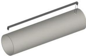
❑ 15. Wrap masking tape around the engine tube about 1" from the bottom to hold the engine hook in place and centered along its length.
