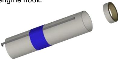
❑ 17. Place two marks on the side of the engine mount, one mark 3/8" from the bottom of the tube and one mark 2-1/4" from the bottom of the tube.
