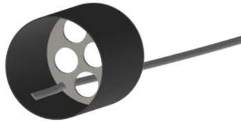
□ 29. Test fit the ejection baffle in the main tube. Sand the edges so it will slide freely in the tube. Apply a bead of glue about 4" inside the top of the main tube. Orient the baffle assembly so the baffle and elastic cord are at the top end. Slide the ejection baffle in the tube past the bead of glue until the top of the baffle is about 4" from the top of the tube. Rotate the main tube as the glue is drying so it does not pool in one place. Allow to dry completely.
