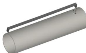
7. Wrap masking tape around the center of the engine tube to hold the engine hook in place and centered along its length.
