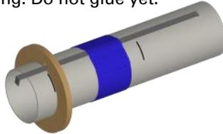
❑ 19. Select the last ring and slide it over the top of the engine mount with the small notch aligned over the engine hook until the second mark at 2-1/4" is just showing. Do not glue yet.
