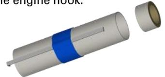
9. Place two marks on the side of the engine mount, one mark 3/8" from the bottom of the tube and one mark 2-1/4" from the bottom of the tube. Place identical marks on the opposite side of the tube. Make another engine mount identical to this one.
