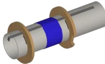
❑ 20. Using the small basswood strip again, test the spacing between the rings. They should almost touch both ends of the strip all around the mount. Adjust the rings, if necessary, and apply glue at the intersection of the tube and rings, keeping glue away from the outer surfaces of the rings and away from the engine hook slot on the bottom ring. Apply a bead of glue over the masking tape at the area over the engine hook. Allow to dry, checking the fit with the basswood strip.
