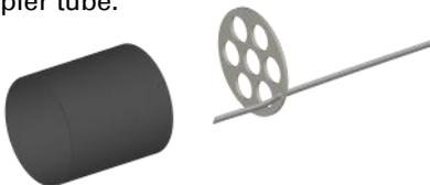
□ 28. Apply a generous bead of glue inside the coupler tube against the joint between the baffle ring and
