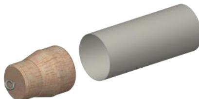
□ 32. Insert the nose cone (BC-2025) into the payload tube and check for fit. A small amount of sanding may be necessary. Make sure it is tightly fitted, using masking tape if necessary. If a payload is added, screws or external tape may be required to secure the nose cone in flight.
