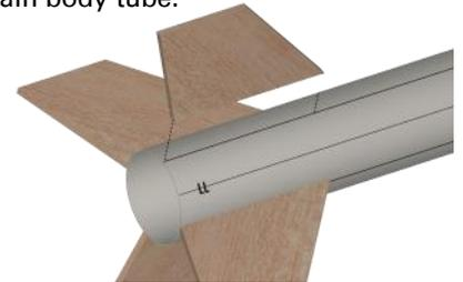
❑ 23. Apply a thick bead of glue on one side of the basswood strip (FV-39S). Glue it on the inside of the main body tube over one of the fins and 1/4" from the bottom of the tube. Make sure it is parallel with the main body tube. Wipe any excess glue from the exposed edges.
