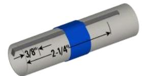
10. Carefully remove the four centering rings from the laser-cut plywood sheet (CR-KV-39). Select the one with two engine mount holes and no slot on the outer edge. Insert the bottom of one of the mounts in one of the small openings. Align the small notch over the engine hook. Slide it from the bottom of the engine tube until the mark at 3/8" is just showing. Add the second engine mount tube in the second hole in a similar manner. Do not glue yet!
