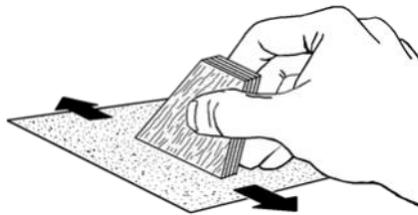
4. Round all the edges of each fin, except leave the root edges flat. Repeat for all six fins. The root edges will be glued to the body tube.
