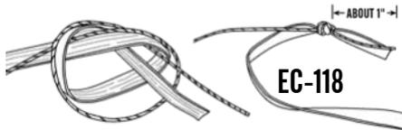
❑ 20. Assemble the chute (CP-12RY) using instructions provided with it. Pull the lines tight on the chute and make sure they are all of equal length. Attach the chute by tying them to the screw eye. Put a drop of glue on the joint to keep the lines from moving. Attach the free end of the elastic cord to the screw eye. Put a drop of glue on that joint as well.
