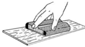
3. Stack all the like fins in sets. Line each set of fins up squarely and sand the fins back and forth over some fine sandpaper to get rid of the hold-in tabs as shown below.
