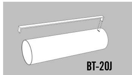
7. Apply a bead of glue inside the punched end of the engine tube. Insert one of the engine blocks (EB-20A) inside the engine tube and flat against the engine hook. After the ring is in place, run a bead of glue around the inside of the ring to protect it from the ejection gases.
