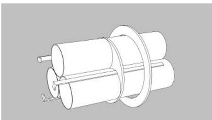
❑ 12. Ball up a small piece of tissue and insert it into the central area between the three tubes. Seal it with a drop of glue to block the exit from the ejection gases.
