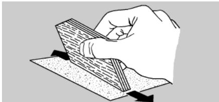
4. Round all the edges of each fin, except root edge which should be left flat to be glued to the body tube. Sand both sides until they are smooth.
