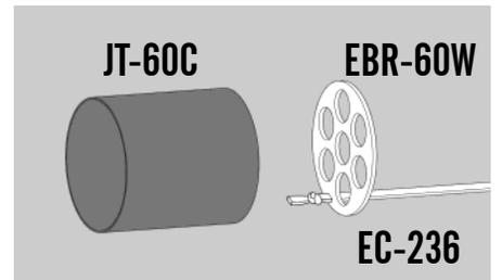
❑ 16. Apply a generous bead of glue inside the coupler tube against the joint between the baffle ring and the coupler tube. Glue the end of the elastic cord to the coupler tube.
