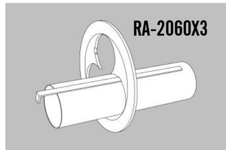
❑ 9. Make a second engine tube assembly repeating steps 5 through 7. Add the second assembly in another hole in the centering ring, aligning the engine hook in the notch as before. Align the end of the engine tube with the first engine tube.
