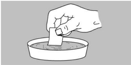
❑ **30.** Slide the decal in place and use the paper backing to work the bubble out. Repeat for all the decals. Be careful with covering decals with a clear coat. Many of the new sprays are not compatible. Future floor polish is suggested.
