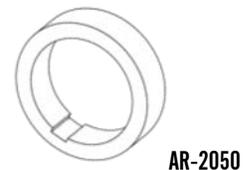
9. Slide an adapter ring from each end until they just touch the marks drawn in a previous step. Apply a bead of glue around each end of the joint between the ring and engine tube, keeping glue off the outside surface of the centering ring. Allow to dry. Tuck the Kevlar® cord inside the engine tube. Set this aside for later. This will be the upper stage mount (with Kevlar). **Make an identical mount for the booster without the Kevlar shock cord.**
