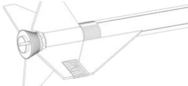
❑ 25. After the fin assembly is completely dry, run a very small bead of glue along both sides of each fin-body tube joint. Using your forefinger, smooth the glue into fillets. Separate the two sections. Wipe any excess glue and allow to dry.
