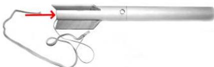
**13.** Attach chute (O) by passing the lines through the screw eye and looping them over the tip of the nose cone. Pull the lines tight and make sure they are all of equal length. Put a drop of glue on the joint to keep the lines from moving. Tie the loose end of the elastic cord to the screw eye. Put a drop of glue on the knot to keep it from untying.
