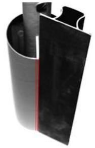
**19.** Prepare the outer fins (G) by sanding the leading and trailing edges round. Using CA glue, tack each outer fin in place with the trailing edge even with the bottom of the shroud tube.
