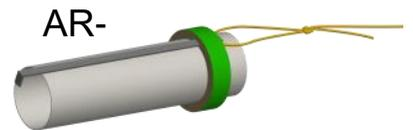
11. Mark 1" from the bottom of the engine mount tube and slide the other centering ring (AR-2050) from the bottom until the bottom of the ring is even with the mark. Run a bead of glue around each side of each ring against the engine tube. Keep glue away from the green outside surface. Allow to dry.
