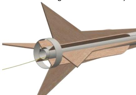
❑ 18. Slide the remaining ring tube (RT-70) over the top of the heatsink fins. Sanding may be necessary to achieve a good fit. Align it until it touches the leading edge of each of the main fin assemblies. Apply a fillet of glue against each heatsink fin where it touches the ring tube. Allow to dry.
