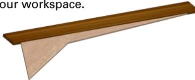
5. Round all the edges of each fin, except the root edges. Leave them flat. Repeat for all eight fins. The root edges will be glued to the body tube.
