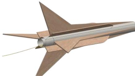
❑ 17. Slide one of the ring tubes (RT-70) over the bottom of the heatsink fins. Sanding may be necessary to achieve a good fit. Align it until it touches the bottom of each of the main fins. Apply a fillet of glue against each heatsink fin where it touches the ring tube. Allow to dry.
