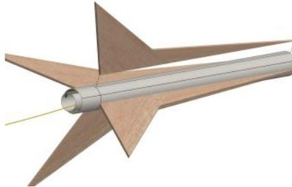
❑ 16. Apply glue to the root edge of one of the long heatsink fins and position it along one of the long lines drawn for the fins on the side of the body tube and even with the bottom of the tube. Use the same techniques used on the main fin assemblies and repeat for the other three heatsink fins. Allow the fins to completely dry, checking carefully to make sure they are parallel with the main body tube.
