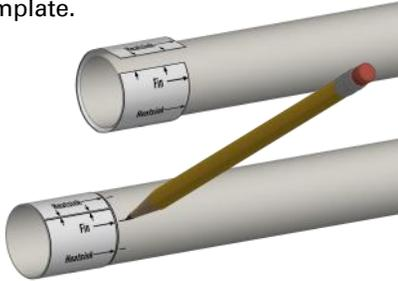
❑ 13. Find a convenient channel or groove such as a partially open drawer (as shown), a door jamb or a piece of molding. Using the channel, extend the marks the full length of the tube for every other mark. Extend the other four marks from the marked ring to the top of the tube.
