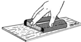
**3.** Stack all the fins in two sets of four. Line the set of fins up squarely and sand the fins back and forth over some fine sandpaper to get rid of the hold-in tabs as shown below.
