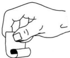
**32.** Mounting the sustainer engine: Apply a piece of masking tape near the bottom of the sustainer engine and install it into the sustainer. Upper stage engines should be long delay. The upper stage may also be flown as a single stage.
