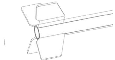
❑ 18. Apply the booster fins in the same manner. They should also be aligned with the bottom (nozzle) end of the booster assembly. Allow both assemblies to dry in a vertical position, checking for proper alignment while drying.
