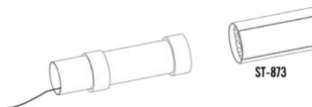
❑ 16. Insert the engine mount in the sustainer body tube until the ends are flush. Rotate the assembly until the glue has flowed around the rings uniformly. Set it on the end until it is completely dry.
