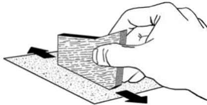
**4.** Round the leading and trailing edges of each fin. Leave the tip and root edges flat. Repeat for all eight fins. The trailing edge can be sanded to a bevel for a more aerodynamic shape.
