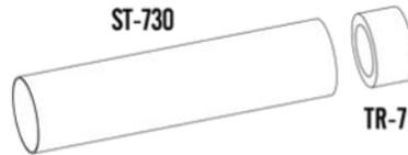
❑ 13. Tie a large knot in one end of the Kevlar thread. Feed it through a centering ring (CR-78) and glue the ring on the engine tube assembly even with the same end with the thrust block. Glue the remaining centering ring 3/4" from the opposite end of the engine tube. Apply generous fillets around each ring.
