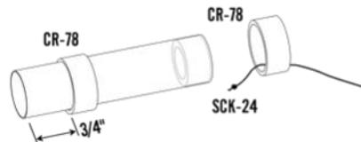
❑ 14. Make sure the Kevlar knot is secure and pulled against the top centering ring. Allow to dry.
