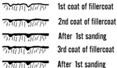
**27.** After all balsa surfaces have been prepared, wipe off all balsa dust with a dry cloth. First spray the model with an enamel primer. Choose a high visibility color like white for the final color.
