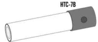
**7.** Glue one centering ring (CR-78) 1/16" from the tube coupler. Glue another centering ring (CR-78) on the opposite end leaving 11/16" of the engine tube exposed. Apply a fillet of glue around the centering rings.
