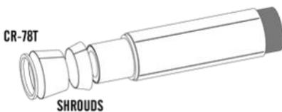
❑ 11. Repeat with the larger shroud. The fiber ring (CR-78T) completes the assembly. Slide it over the engine tube and against the larger ring. Allow to dry.
