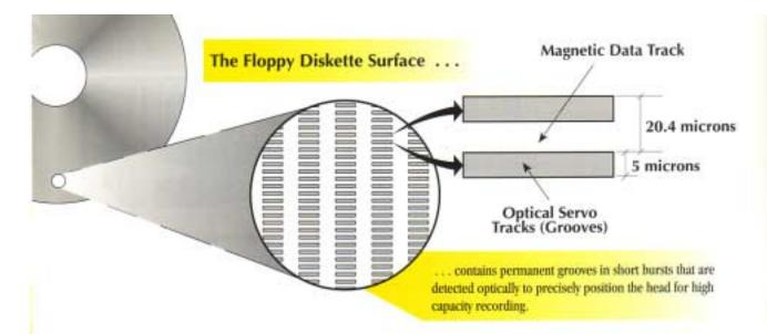
laser etches each of the servo marks as the disk spins. This process ensures an optical pattern for high contrast while maintaining a smooth surface. At the same time, this process allows for the magnetic reference track to be located on the diskette with very high accuracy using the laser guidance system. With laser etching, every diskette is essentially a master. Floptical diskettes from all approved manufacturers, whether stamped or laser etched, are capable of working in any Floptical drive.
