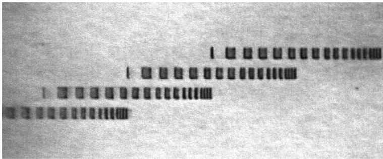
**Figure 6. A disk indelible utility mark on Pocket Zip flexible media. DIUM creates an unalterable media serial number that a drive's magnetic head can read but not replicate.**
