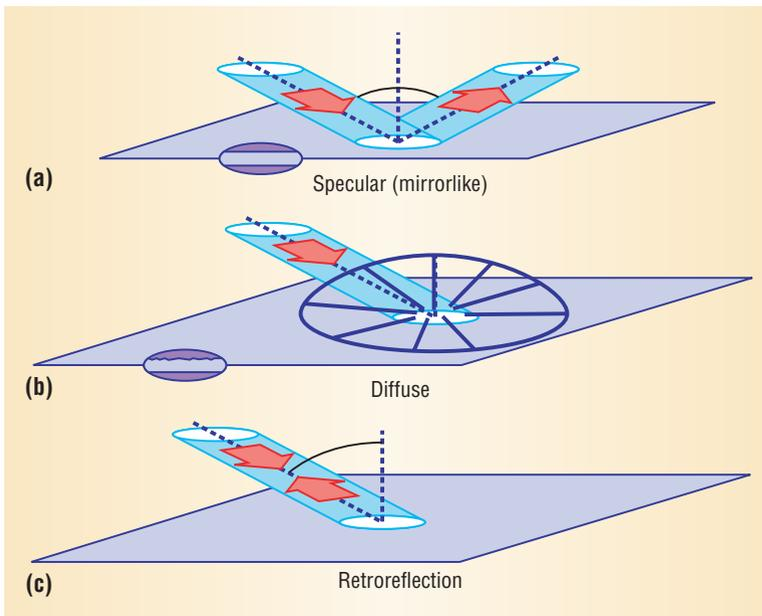
**Figure 1. Principal types of reflection contrasted: (a) specular (mirrorlike), (b) diffuse, and (c) retroreflection.**
