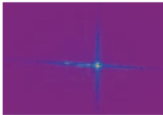
**Figure 4. Reflected irradiance pattern for X-LSD holographic cartridge tag. The point at which the axes cross is the illuminating LED's location.**
