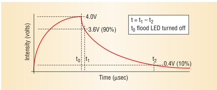
**Figure 5. Typical temporal signal profile of a latent-irradiance material. The detection circuitry for this signal can implement automatic gain control (AGC) techniques. These implementations provide a significant level of system measurement robustness with varying signal amplitude.**
