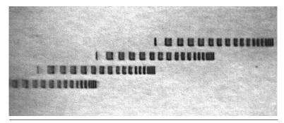
Figure 6. A disk indelible utility mark on Pocket Zip flexible media. DIUM creates an unalterable media serial number that a drive's magnetic head can read but not replicate.
