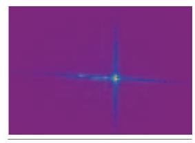
Figure 4. Reflected irradiance pattern for X-LSD holographic cartridge tag. The point at which the axes cross is the illuminating LED's location.
