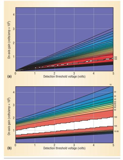
Figure 3. (a) Single-detector cartridge discrimination performance (retrotag versus specular reflector). (b) Dual-detector cartridge discrimination performance (retrotag versus specular reflector).
