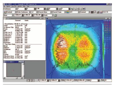
Figure 2. Reflective irradiance pattern of Zip 100 retrotag. The reflected irradiance in the structure is brightest in the hexagon's lobes where the photosensitive detector is placed.
