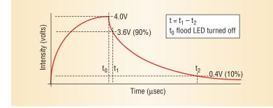
Figure 5. Typical temporal signal profile of a latent-irradiance material. The detection circuitry for this signal can implement automatic gain control (AGC) techniques. These implementations provide a significant level of system measurement robustness with varying signal amplitude.
