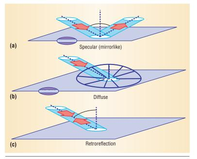
Figure 1. Principal types of reflection contrasted: (a) specular (mirrorlike), (b) diffuse, and (c) retroflection.
