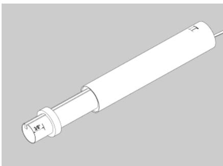
**15.** Pull the long end of the elastic cord taut until the knot is seated against the top slit. Apply a bead of glue on the knot and on the part of the elastic cord that is exposed on the outside of the insulating tube. Wipe any excess glue from the outside of the insulating tube. Store the excess length of the elastic cord inside the insulating tube.
