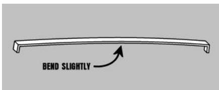
6. Insert one end of the engine hook into the pre-punched engine tube (ST-730E).
