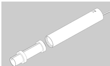
**14.** Mark the engine mount 3/8" from the bottom of the engine tube.
