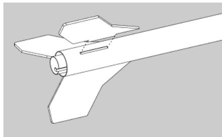
**19.** As the fins are drying, use the laser-cut fin template to align the fins perpendicular to the main body tube. The template will work with three or four fins. Turn it until the three fins line up with the corresponding slots. Do not let any glue set with the template in place.
