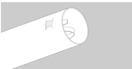
**16.** Insert the insulating tube and engine mount assembly into the main body tube (ST-10100S3) until the lower centering ring is just outside the main body tube. Align the engine hook between two of the slots. Apply a heavy bead of glue around the top side of the lower centering ring.
