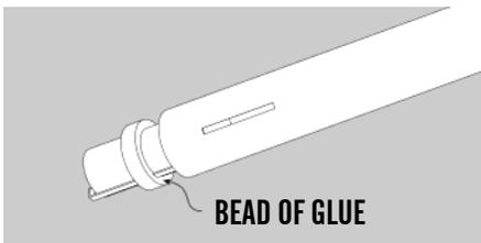
**17.** Push the engine mount into the main body tube until the mark on the engine tube is even with the main body tube. Hold the assembly vertical with the engine mount downward. Make sure all the slots are free of glue while the assembly sets.
