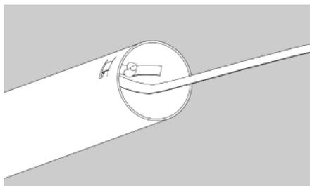
**13.** Apply a bead of glue inside the bottom of the insulating tube (away from the elastic cord.) Insert the engine mount into the insulating tube until it is recessed about 1/16". Roll the assembly on a flat surface to make sure it is aligned properly.
