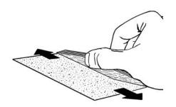
17. Round all edges except the root edge. The root edge should remain flat since it will be glued to the body tube.
