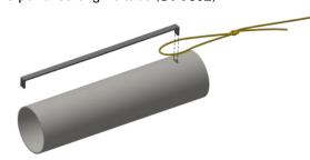
□ 9. Carefully remove the two centering rings from the laser-cut set (CR-7-55EH). Select the one with the small notch and align the notch over the engine hook, Slide it from the bottom of the engine tube until it is against the end of the engine hook and against the yellow Kevlar® cord.
