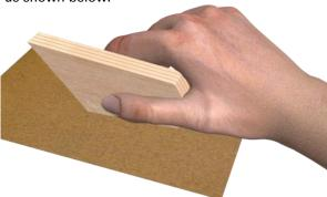
□ 4. Round all the edges of each fin, except the root edges. Leave them flat. Repeat for all four fins. The root edges will be glued to the body tube.
