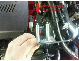
Bolt the cover in place. Start by hand threading the screws in. The cover has a little bit of adjustment room so make sure it is sitting straight and finish by tightening with a 5mm allen wrench until snug.
