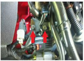
Make sure the ground wire stays in place (red arrow) while bolting the cover onto the fuel pump housing.
