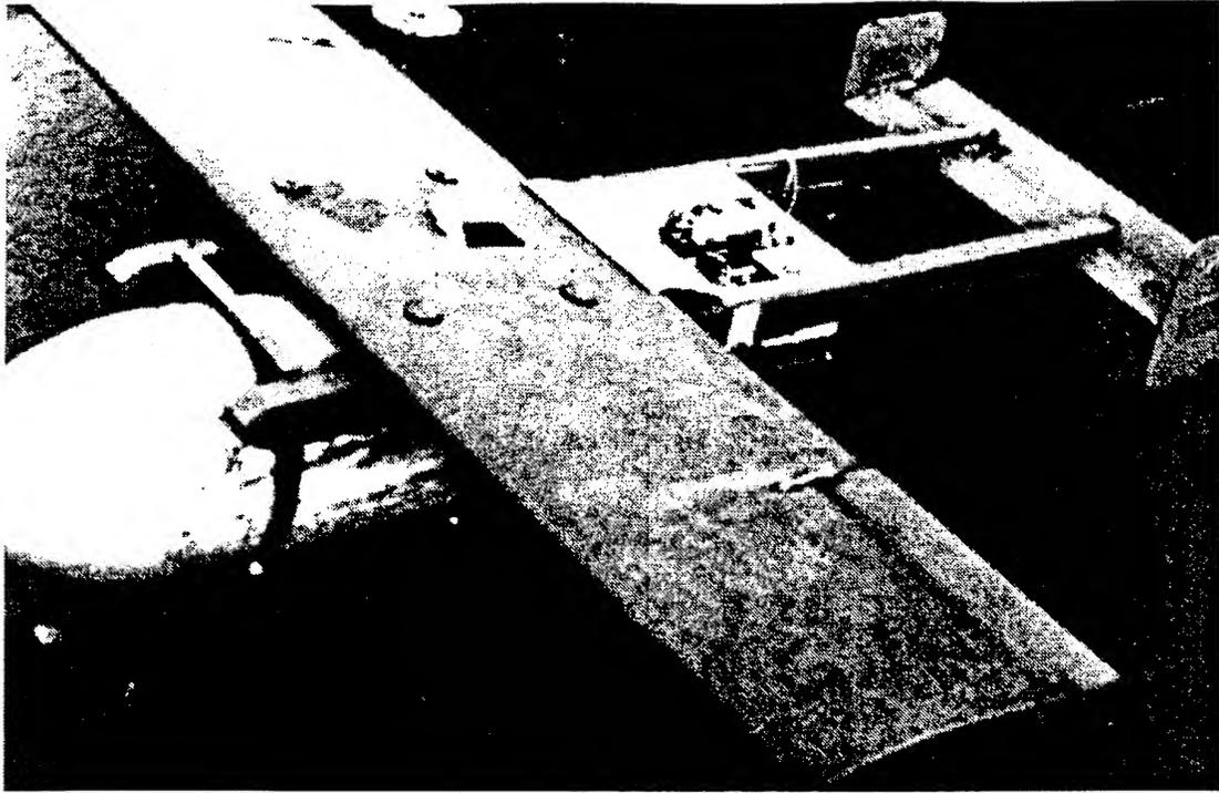
49. The GB-1 was specifically designed to keep aircraft away from enemy flak belts. Two were loaded on specially modified B-17s and, although ineffective, were a stepping stone to "smart bombs" (USAF Museum)
