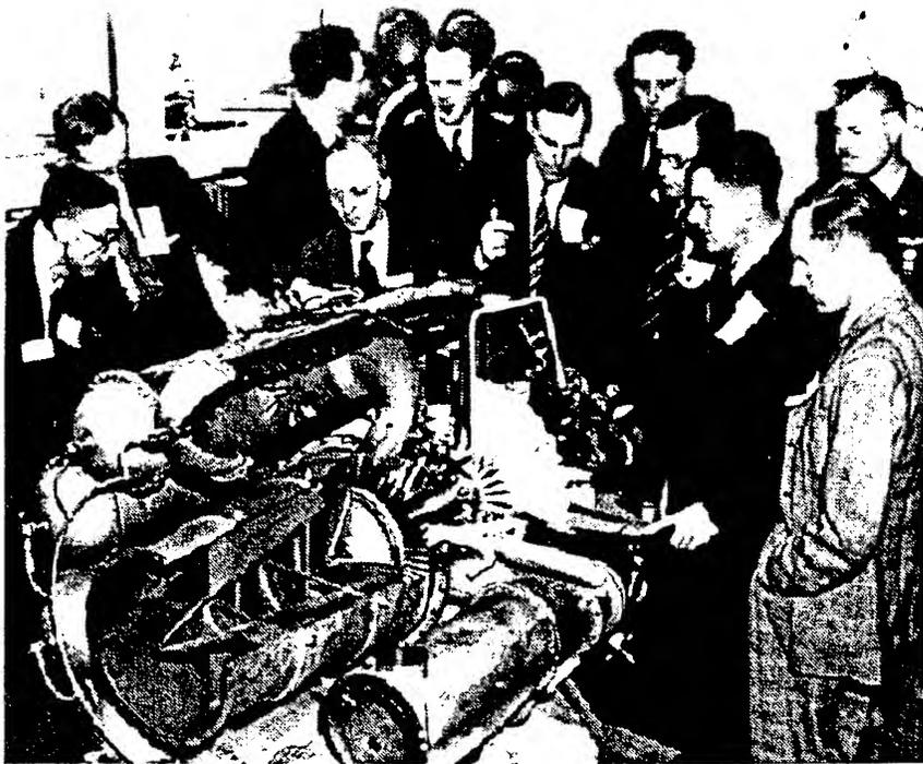
43. The British get a look at their modified Whittle engine, the A-1. GE engineers made a few modifications to the original design which increased efficiency. (Courtesy AFMC/HO, from the GE Collection)
