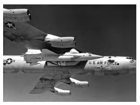
B-52 mother ship with X-15A-2. The latter mounted a dummy scramjet and carried external tanks as well as ablative thermal protection. (NASA)
