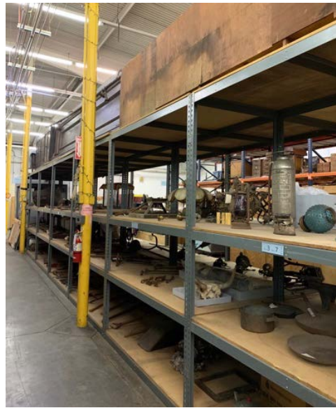
Figure 9: Detail of current open shelving storage with smaller objects on the bottom and large objects on top. Glass items are on higher shelves, but there is no netting or protection to keep objects from coming off of shelves in a seismic event. Shelves are mechanically fastened between units along the length of the rows.
