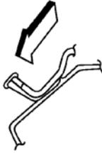
HOLD GUN NOZZLE IN DIRECTION OF ARROW IN ORDER TO EFFECTIVELY SEAL METAL JOINTS.
