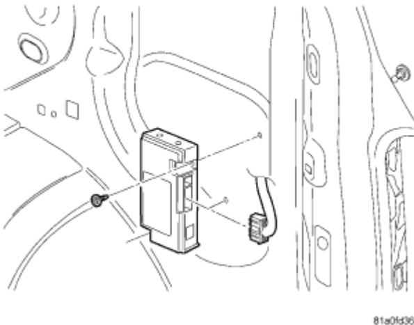
**Fig. 2: Installing Hands Free Module**
