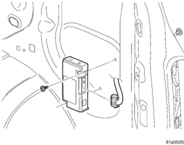
**Fig. 1: Removing Hands Free Module**
