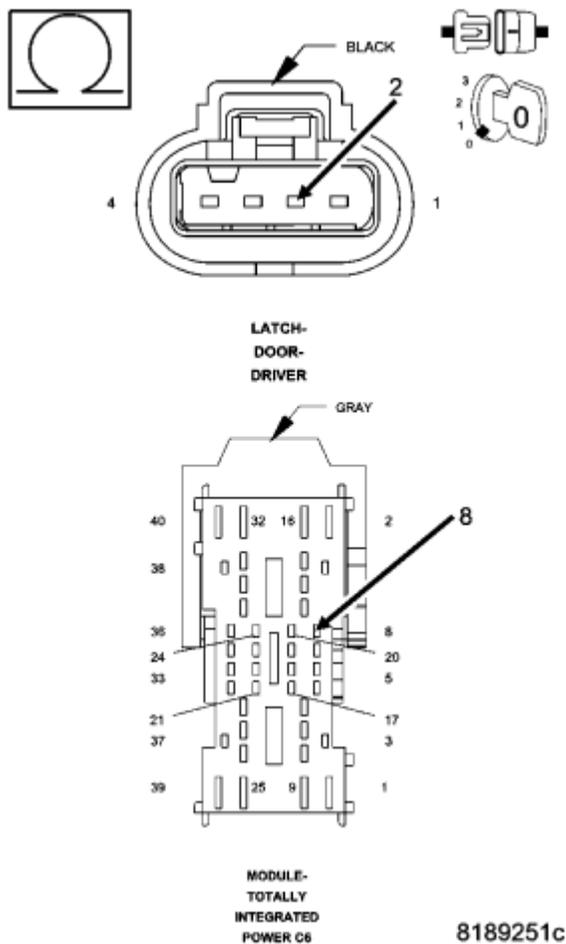
**Fig. 44: Measuring Resistance Of (P930) Driver Door Lock Driver Circuit Between TIPM C6 Connector And Driver Door Latch Connector**
