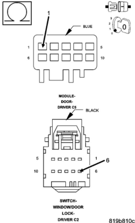
**Fig. 8: Measuring Resistance Of (D500) Lin Bus Circuit Between Door Module C5 Connector And Window/Door Lock Switch Connector**
