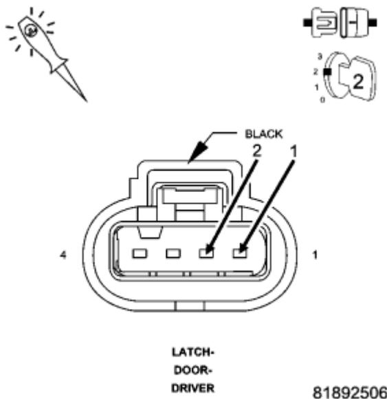
**Fig. 41: Connecting Test Light Between (P930) Driver Door Lock Driver Circuit And (P910) Driver Door Unlock Driver Circuit**
