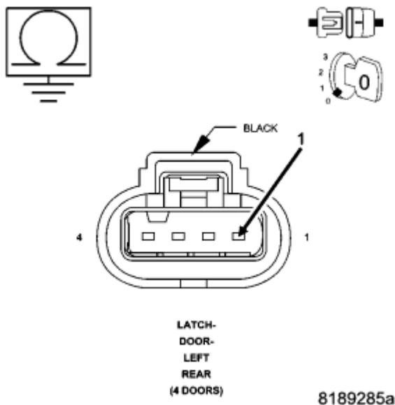
**Fig. 55: Measuring Resistance Between Ground And Appropriate Door Unlock Driver Circuit**
