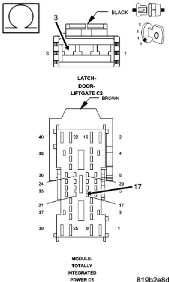
**Fig. 48: Measuring Resistance Of (P306) Tailgate Unlock Driver Circuit Between Latch Connector And TIPM C5 Connector**
