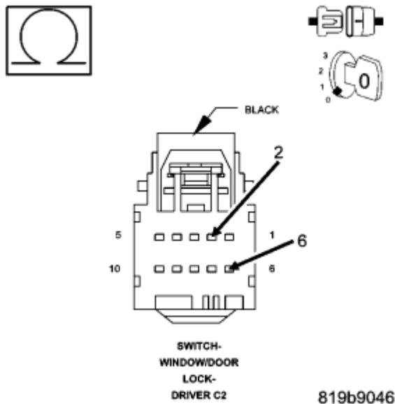
**Fig. 9: Measuring Resistance Between (D500) Lin Bus Circuit And (D501) Lin Bus Return Circuit In Window/Door Lock Switch Connector**
