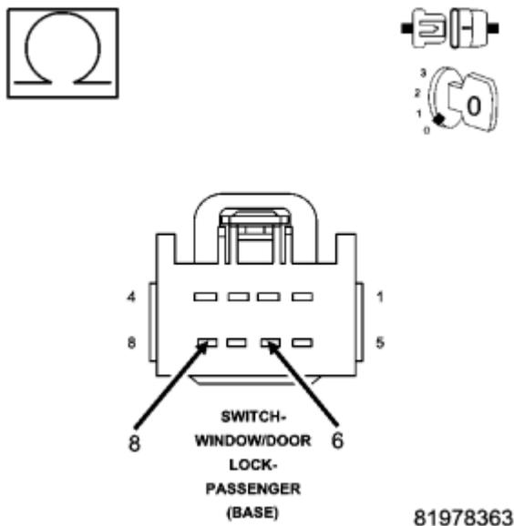
**Fig. 13: Measuring Resistance Between (G160) Passenger Door Lock Switch Mux Circuit And (P37) Door Lock Switch Return Circuit In Switch C2 Connector**
