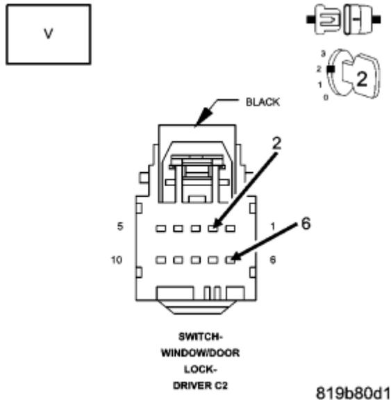
**Fig. 6: Measuring Voltage Between (D500) Lin Bus Circuit And (D501) Lin Bus Return Circuit**
