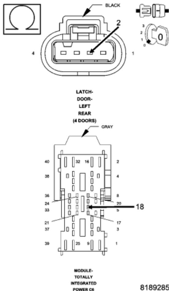
**Fig. 56: Measuring Resistance Of Appropriate Door Lock Driver Circuit Between TIPM C6 Connector And Appropriate Door Latch Connector**
