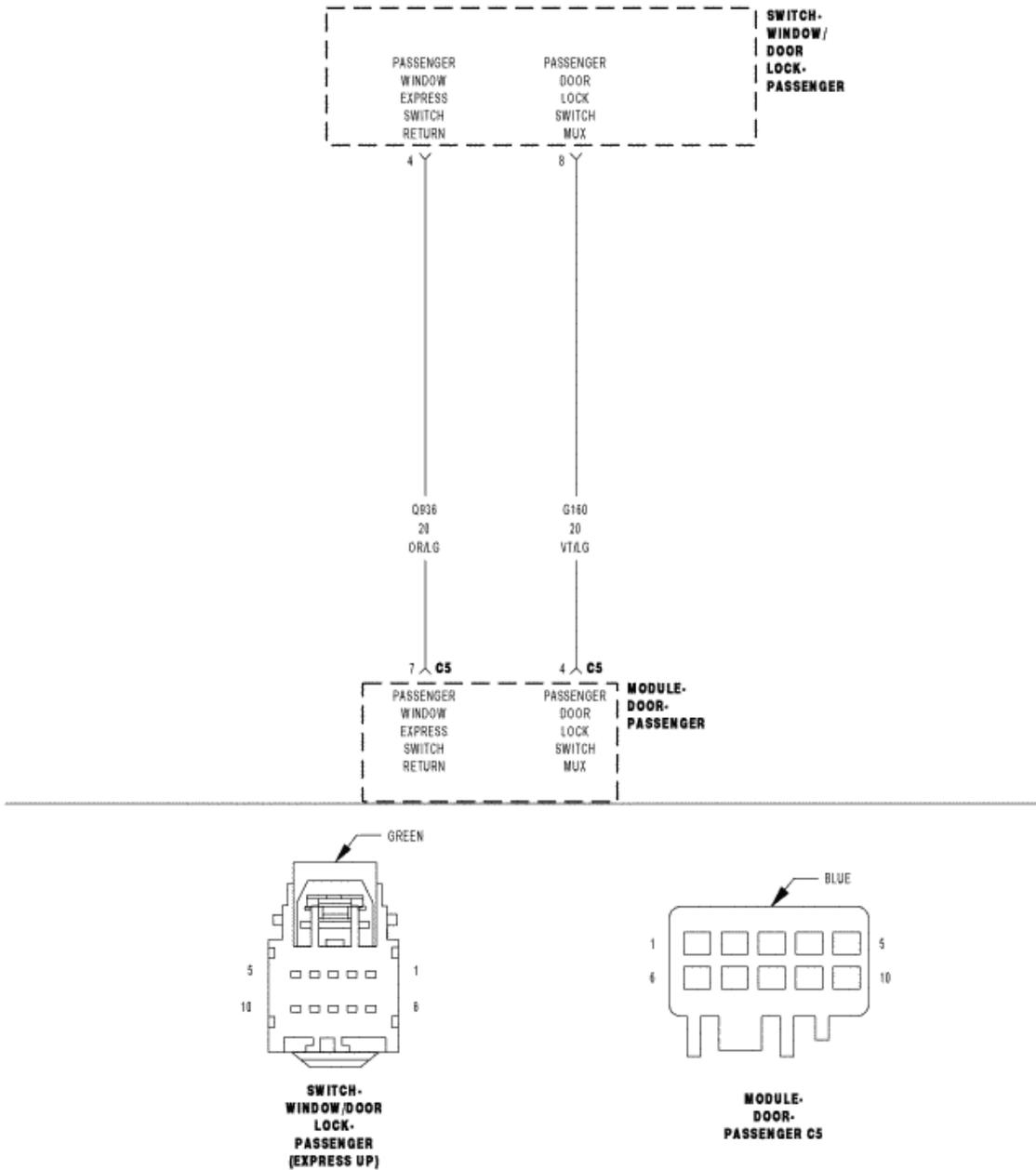
**Fig. 14: Passenger Door Lock Switch Circuit Schematic**
