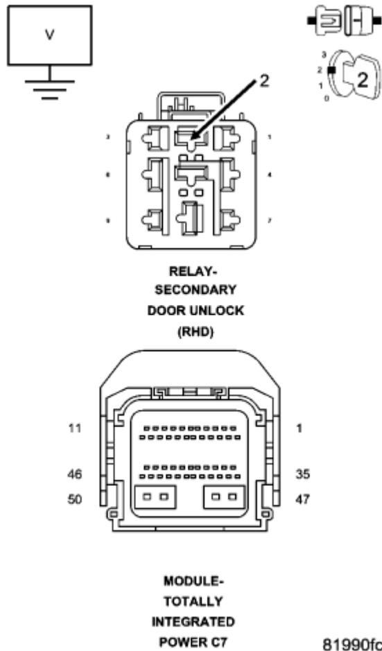
**Fig. 39: Measuring Voltage Between Ground And (P391) Secondary Door Unlock Relay Control Circuit In Relay Connector**
