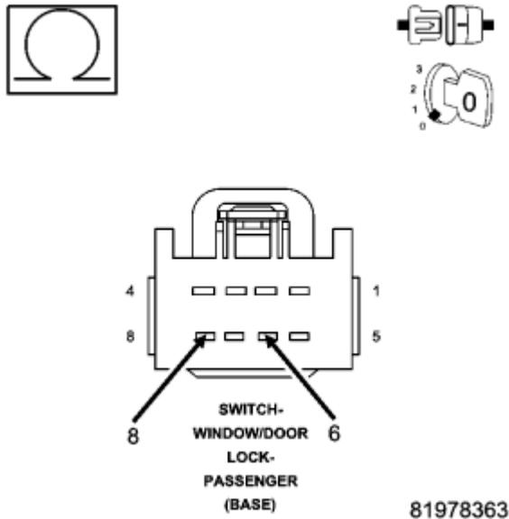
**Fig. 32: Measuring Resistance Between (G160) Passenger Door Lock Switch Mux Circuit And (P37) Door Lock Switch Return Circuit In Switch C2 Connector**
