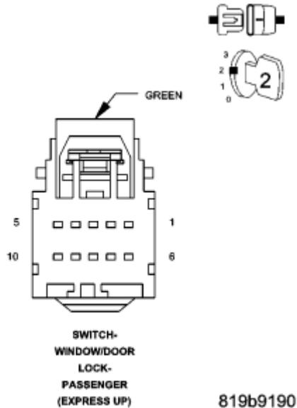
**Fig. 15: Passenger Window/Door Lock Switch Connector**
