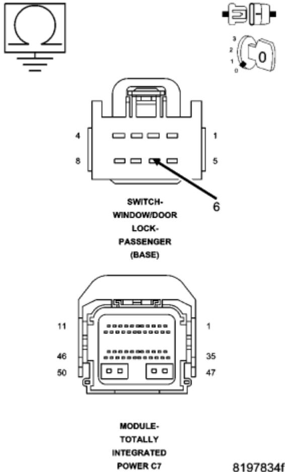
**Fig. 12: Measuring Resistance Between Ground And (G160) Passenger Door Lock Switch Mux Circuit**
