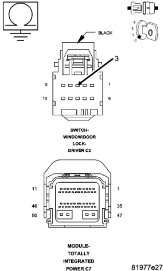
**Fig. 27: Measuring Resistance Between Ground And (G161) Driver Door Lock Switch Mux Circuit In Driver Window/Door Lock Switch C2 Connector**
