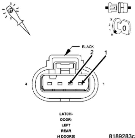
**Fig. 53: Connecting Test Light Between Door Lock Driver Circuit And Door Unlock Driver Circuit**
