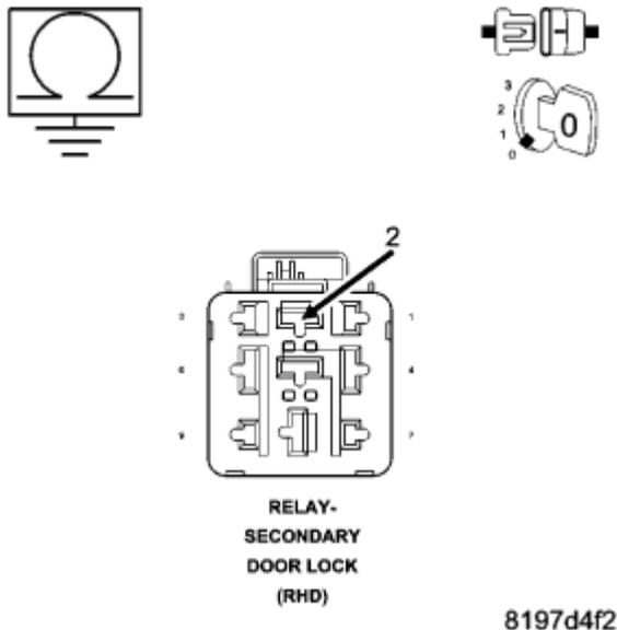
**Fig. 20: Measuring Resistance Between Ground And (P390) Secondary Door Lock Relay Control Circuit In Relay Connector**
