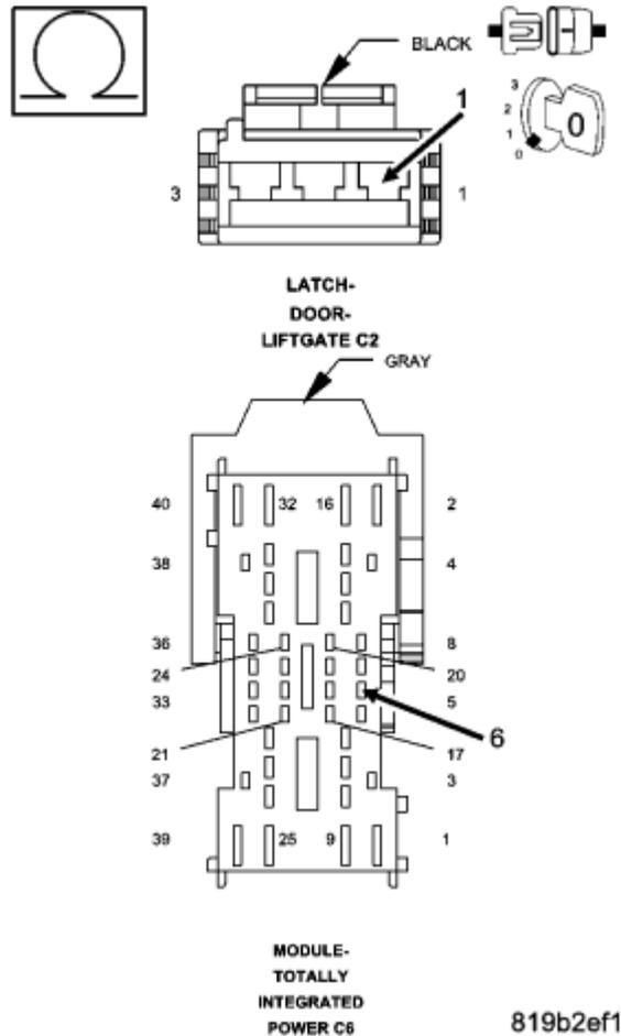
**Fig. 50: Measuring Resistance Of (P304) Tailgate Lock Driver Circuit Between TIPM C6 Connector And Tailgate Latch Connector**
