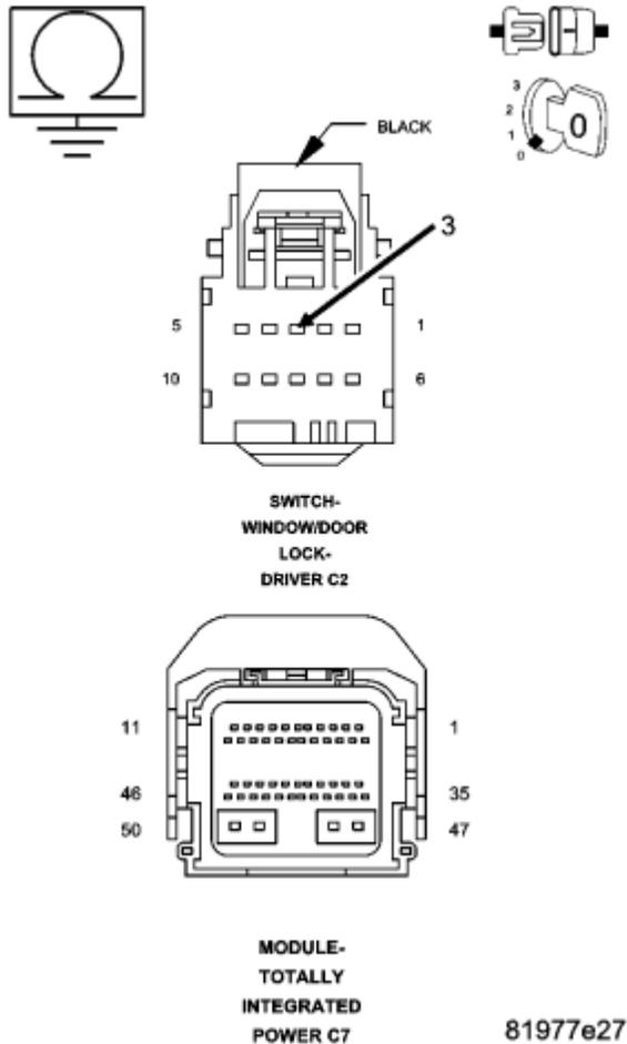
**Fig. 3: Measuring Resistance Between Ground And (G161) Driver Door Lock Switch Mux Circuit In Driver Window/Door Lock Switch C2 Connector**
