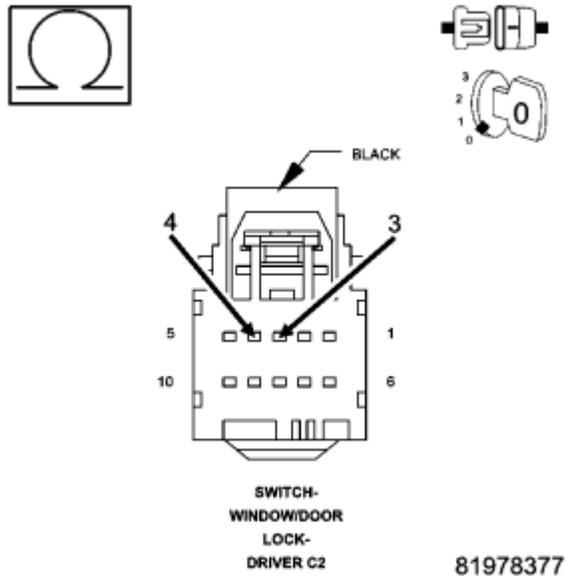
**Fig. 4: Measuring Resistance Between (G161) Driver Door Lock Switch Mux Circuit And (P37) Door Lock Switch Return Circuit In Switch C2 Connector**
