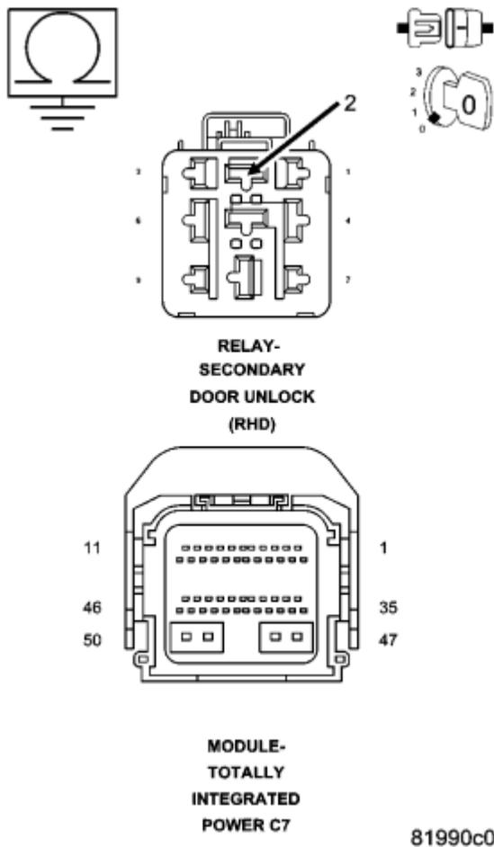
**Fig. 35: Measuring Resistance Between Ground And (P391) Secondary Door Unlock Relay Control Circuit In Relay Connector**
