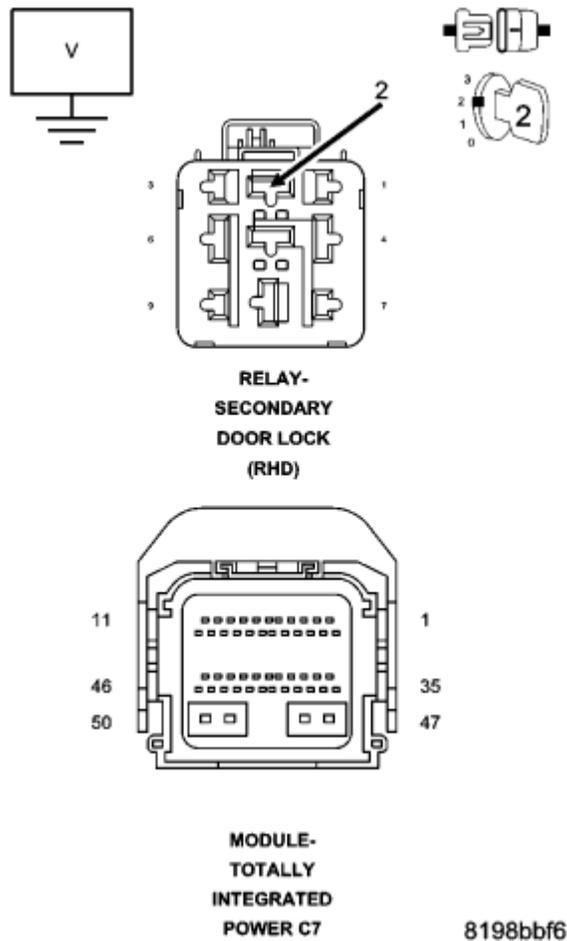
**Fig. 24: Measuring Voltage Between Ground And (P390) Secondary Door Lock Relay Control Circuit In Relay Connector**
