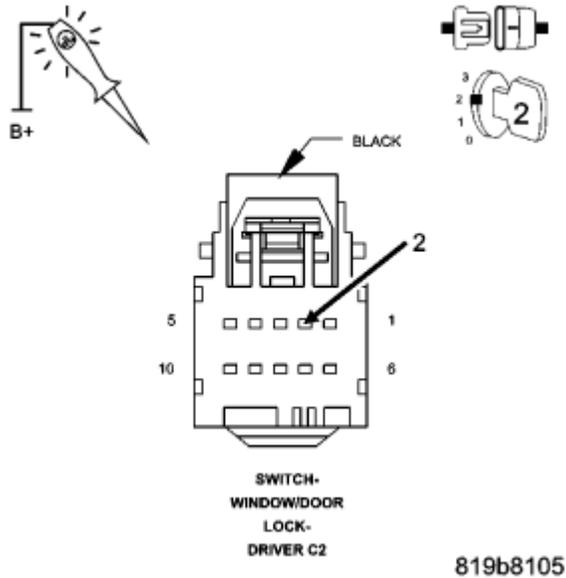
**Fig. 7: Using 12-Volt Test Light Connected To 12-Volts To Check (D501) Lin Bus Return Circuit**
