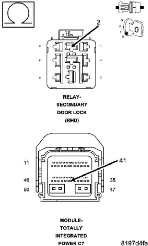
**Fig. 21: Measuring Resistance Of (P390) Secondary Door Lock Relay Control Circuit Between Relay Connector And TIPM C7 Connector**
