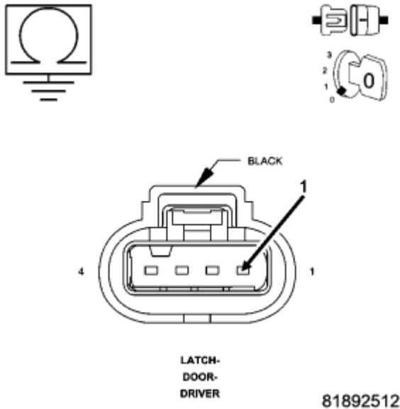
**Fig. 43: Measuring Resistance Between Ground And (P910) Driver Door Unlock Driver Circuit**
