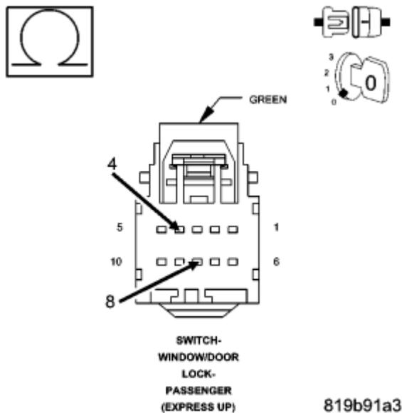
**Fig. 17: Measuring Resistance Between (G160) Passenger Door Lock Switch Mux Circuit And (Q936) Passenger Window Express Switch Return Circuit**
