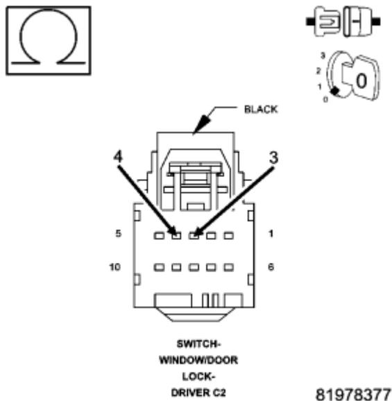
**Fig. 28: Measuring Resistance Between (G161) Driver Door Lock Switch Mux Circuit And (P37) Door Lock Switch Return Circuit In Switch C2 Connector**
