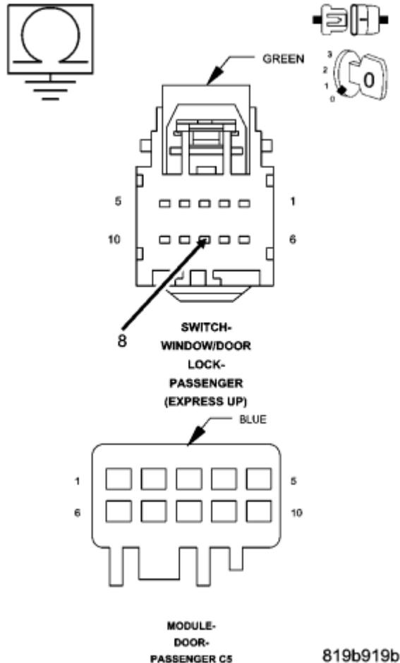
**Fig. 16: Measuring Resistance Between Ground And (G160) Passenger Door Lock Switch Mux Circuit In Passenger Window/Door Lock Switch Connector**
