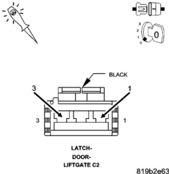
**Fig. 47: Connecting Test Light Between (P304) Tailgate Lock Driver Circuit And (P406) Tailgate Unlock Driver Circuit**
