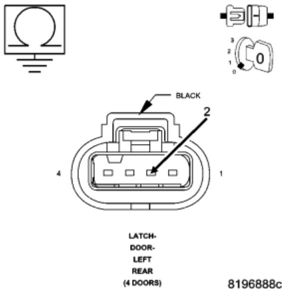
**Fig. 57: Measuring Resistance Between Ground And Appropriate Door Lock Driver Circuit**
