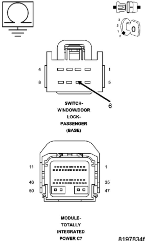
**Fig. 31: Measuring Resistance Between Ground And (G160) Passenger Door Lock Switch Mux Circuit**
