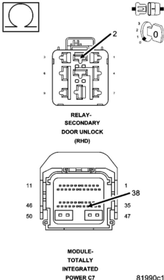
**Fig. 36: Measuring Resistance Of (P391) Secondary Door Unlock Relay Control Circuit Between Relay Connector And TIPM C7 Connector**
