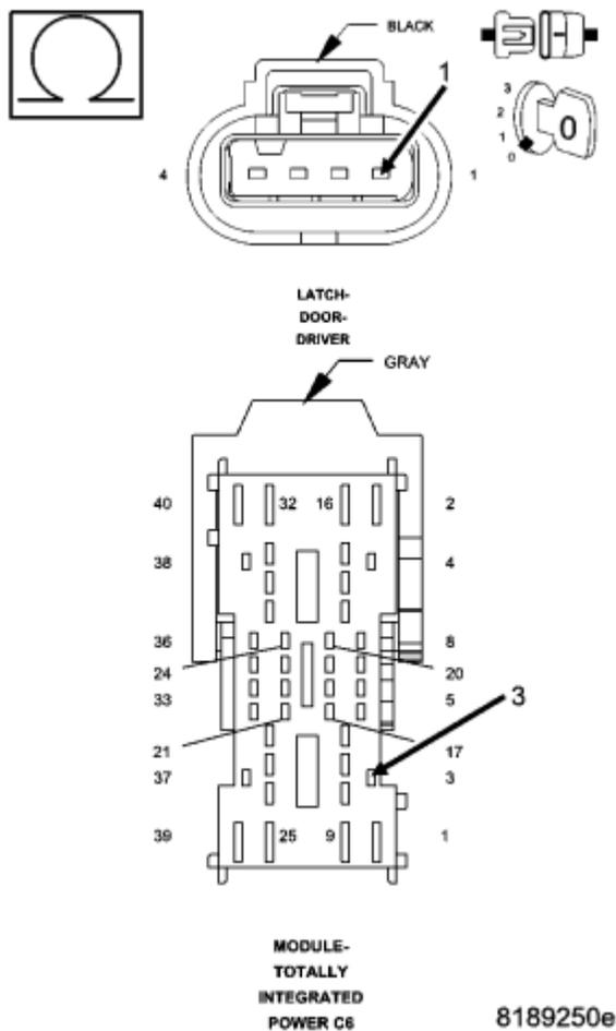
**Fig. 42: Measuring Resistance Of (P910) Driver Door Unlock Driver Circuit Between Latch Connector And TIPM C6 Connector**
