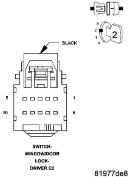
**Fig. 2: Driver Window/Door Lock Switch C2 Connector**
