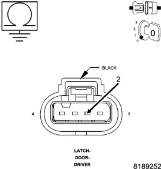
**Fig. 45: Measuring Resistance Between Ground And (P930) Driver Door Lock Driver Circuit**
