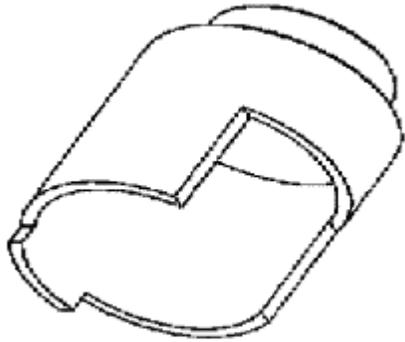
**Fig. 13: Clevis Bushing - 9956**
