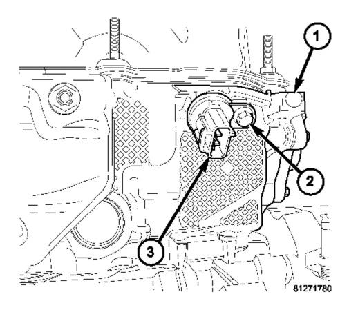
Fig. 3: Identifying Right Cylinder Head, Sensor Mounting Bolt & Camshaft Position Sensor (CMP) Courtesy of CHRYSLER LLC
