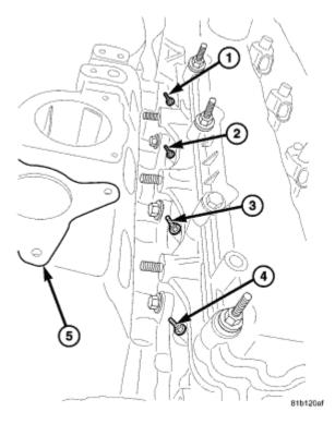
Fig. 33: Glow Plugs - 2.8L Diesel Courtesy of CHRYSLER LLC
