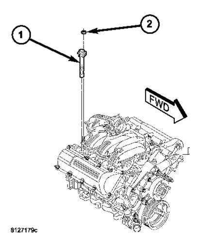
Fig. 12: Locating Ignition Coil - 3.7L Courtesy of CHRYSLER LLC
