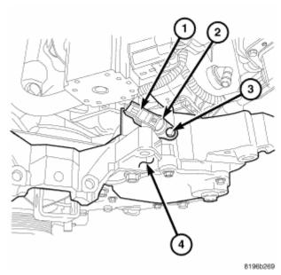
Fig. 5: Identifying CMP Sensor Electrical Connector, Twist Sensor & Sensor Mounting Bolt Courtesy of CHRYSLER LLC
