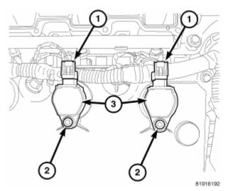
Fig. 13: Identifying Ignition Coil Electrical Connector, Coil Mounting Bolt & Ignition Coils Courtesy of CHRYSLER LLC
