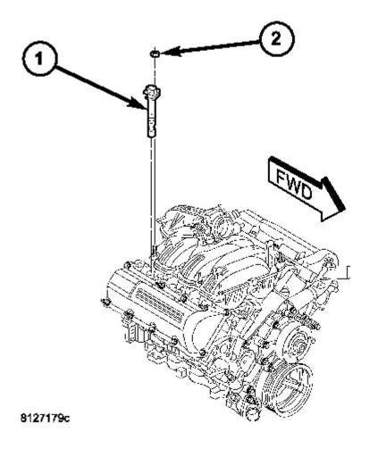
Fig. 9: Locating Ignition Coil - 3.7L Courtesy of CHRYSLER LLC
