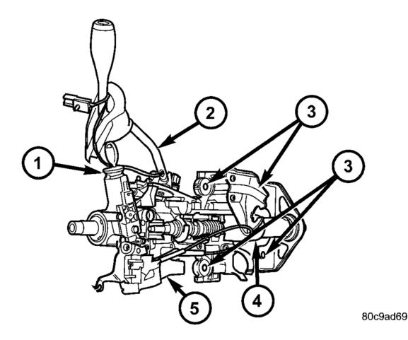
Fig. 19: Identifying Key Cylinder, Gear Shift Lever, Mounting Holes, Steering Column & Ignition Switch Courtesy of CHRYSLER LLC
