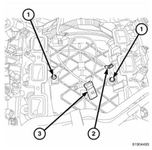
Fig. 14: Identifying Knock Sensors, Identification Tag (LEFT) & Electrical Connector Courtesy of CHRYSLER LLC
