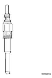
Fig. 30: Glow Plug Courtesy of CHRYSLER LLC
