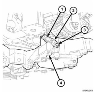
Fig. 7: Identifying CMP Sensor Electrical Connector, Twist Sensor & Sensor Mounting Bolt Courtesy of CHRYSLER LLC
