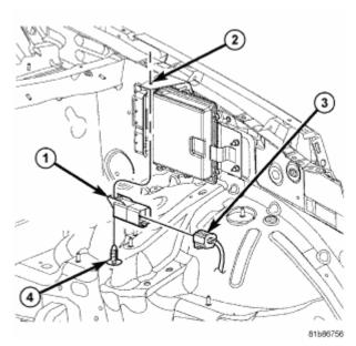
Fig. 36: Identifying Glow Plug Relay (Module), ECM Mounting Bracket, Electrical Connector & Pin Courtesy of CHRYSLER LLC
