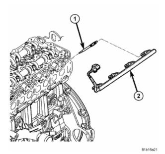
Fig. 35: Glow Plugs & Glow Plug Wiring Harness
