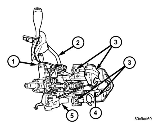
Fig. 18: Identifying Key Cylinder, Gear Shift Lever, Mounting Holes, Steering Column & Ignition Switch Courtesy of CHRYSLER LLC
