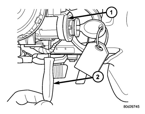
Fig. 28: Key Cylinder & Punch Courtesy of CHRYSLER LLC
