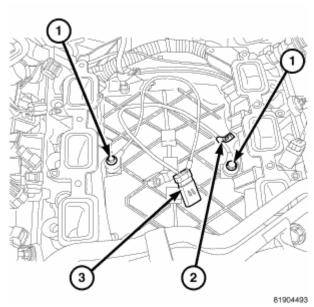
Fig. 16: Identifying Knock Sensors, Identification Tag (LEFT) & Electrical Connector Courtesy of CHRYSLER LLC
