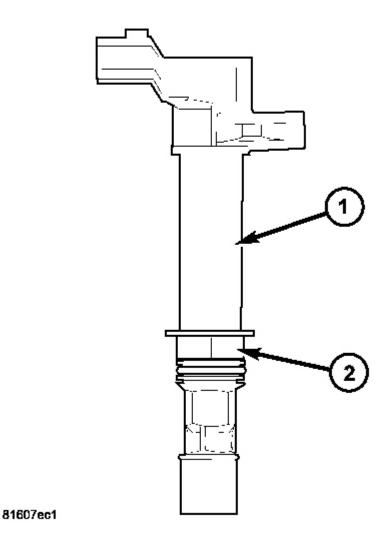
Fig. 8: Ignition Coil Seal & O-Ring Courtesy of CHRYSLER LLC
