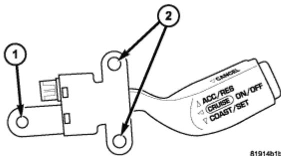
**Fig. 1: Speed Control Switch**
