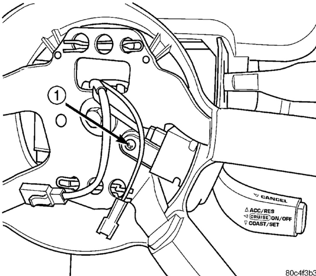
**Fig. 5: Speed Control Switch Mounting Screws**
