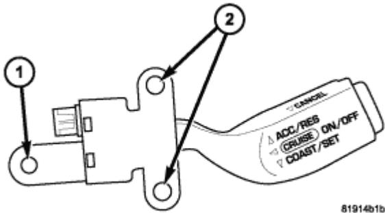
**Fig. 4: Speed Control Switch**
