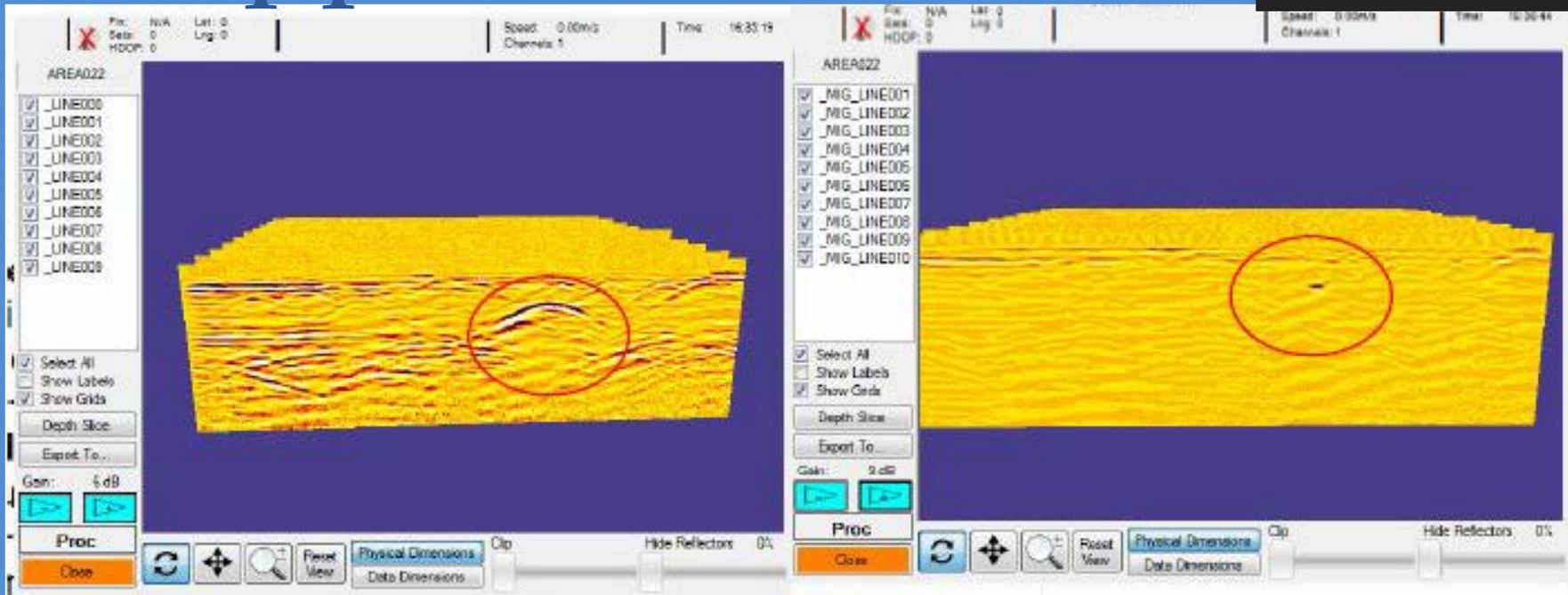
Cross section data must be filtered and hyperbolas corrected to generate 3d bitmap data.
