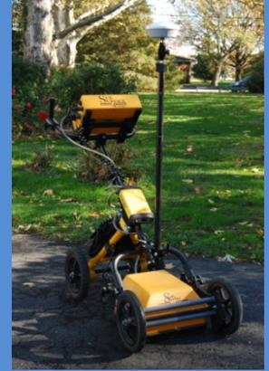
1) Treat the gpr like a data collector using a gps unit and manually select points on the cross-section data in real time in the field.
