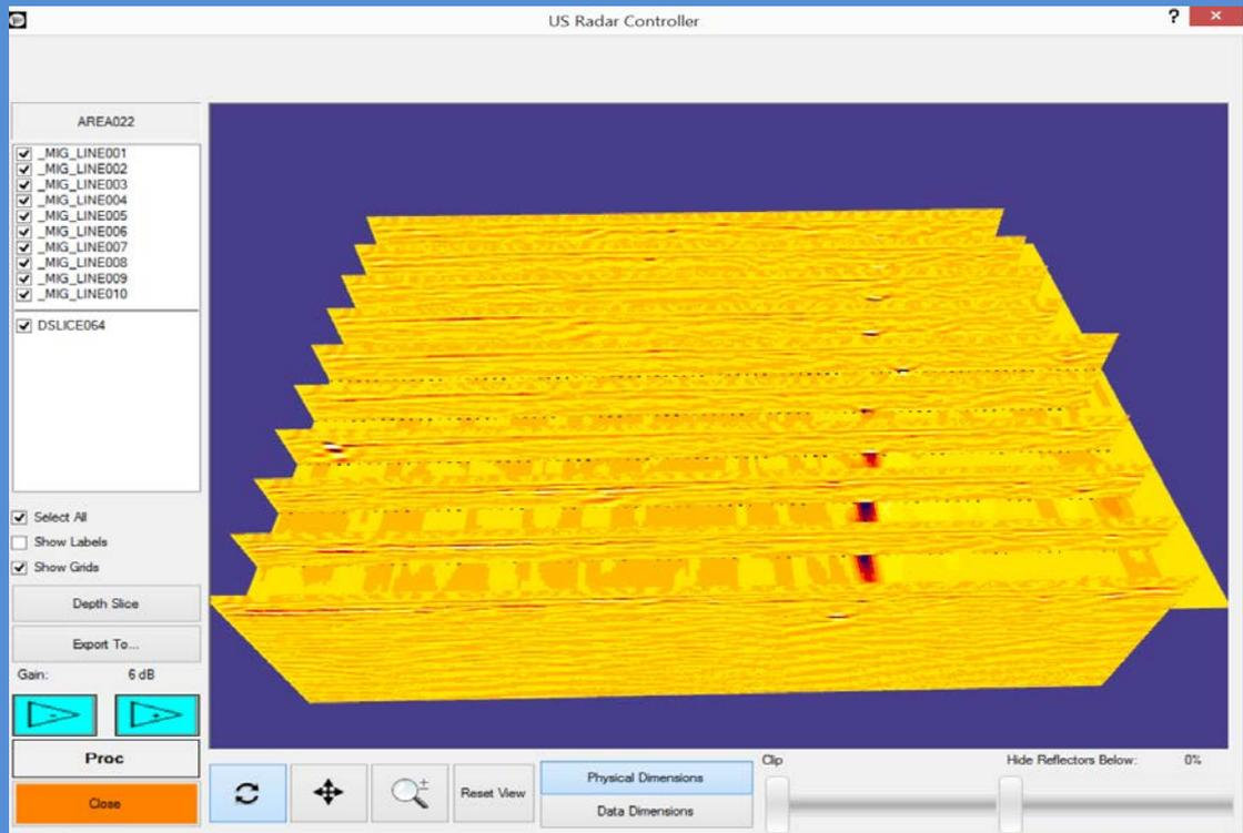
After cross-sections are processed, then an interpolation algorithm connects/stitches the 'blips' from one cross section to the next.
