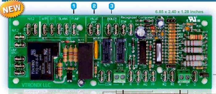
R200 is a microprocessor based control for operating a Combo air handler. It provides control for a two speed line voltage fan motor or low voltage control of an ECM motor, line voltage control of a water pump, 24VAC control of an isolation valve and control of a dry switching relay to turn on/off a water heater.
