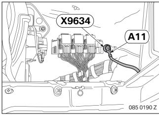
Connect branch **A11** to earth post connection **X9634** in the footwell at the front right.
