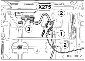
Connect the connection cables (1) of the heated covers for the seat base and backrest under the seat and clip them into the mountings (2).
