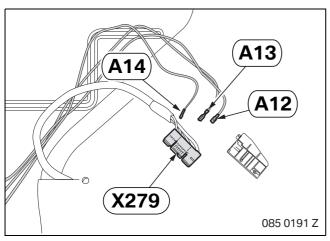
Connect branches **A12 – A14** to passenger's seat plug **X279** as follows:
