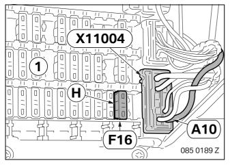
Connect branch **A10** to PIN 1 on plug **X11004** of fuse holder (1).
