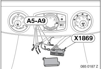
Route wiring harness **A** in the car and attach it to the existing wiring harnesses.
