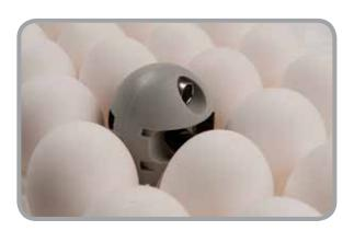
Pilot™ Sensor monitoring egg shell temperature and ambient temperature to send data to Delta Drive™.
