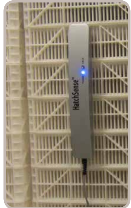
HatchSense™ attached to a stack of plastic hatcher baskets, monitoring eggs to detect when the first birds hatch.
