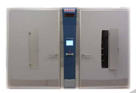
WiseView<sup>™</sup> optional windows on the hatchers include covers to keep light out during hatch cycle. WiseView™ incubator windows are coverless.
