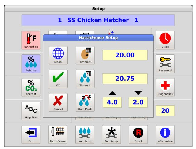
Internal pip timeout sets the day-in-cycle when the profile advances to the pip phase even if chick motion has not yet been detected. This value should be selected such that the profile has sufficient time to complete the pip steps before the humidity level starts to peak, otherwise the humidity phase may not have enough time to finish. This number also selects the point where regular setpoint steps appear above or below the HatchSense block.
