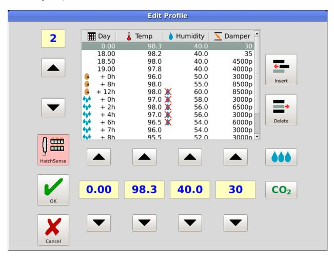
When the HatchSense button is in highlighted state, the profile will be saved as a HatchSense mode profile, otherwise it will be saved as a standard profile.
