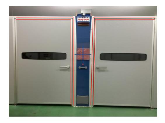
Adjust the door so that the console-door gap is equal top to bottom.
