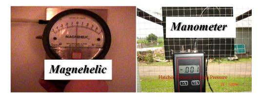
The preferred instrument for proper monitoring the Jamesway Incubator Cabinet Pressure is the digital Manometer as shown. A proper Magnehelic can be used but must be the scale as shown and must leveled and zeroed for accurate reading.
