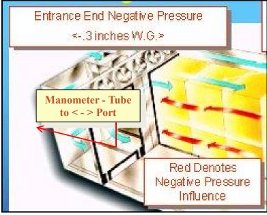
The second incubator pressure check is entrance end negative pressure. While still in the entrance end of the incubator take the tube and run it under the threshold at the track into the hall. Put the tube on the negative (-) port of the instrument. This reading must be 60% of the total i.e. @ .50 inches W.C. total incubator pressure the correct entrance end pressure is <-.30> inches W.C.
