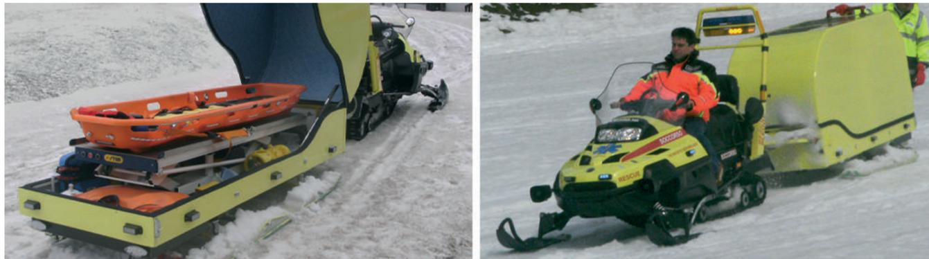
"Snow Ambulance" was designed to transport critically ill patients on snow-covered slopes. The patient transport shell is equipped with a shock-absorbing stretcher support and heating system. In addition, Snow Ambulance is provided with the equipment and devices necessary for first aid. A window has been installed in the upper part of the lid to ensure greater patient comfort and monitoring by the doctor during transport.
