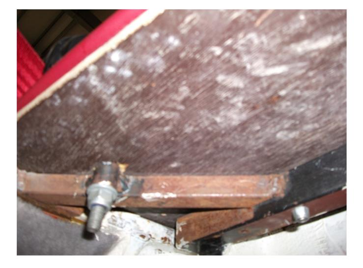
In the first image the seat belt anchorage point looks securely bolted from above but, as shown in the second image, underneath the seatbelt bolts to a frame that is secured to wooden panels.
