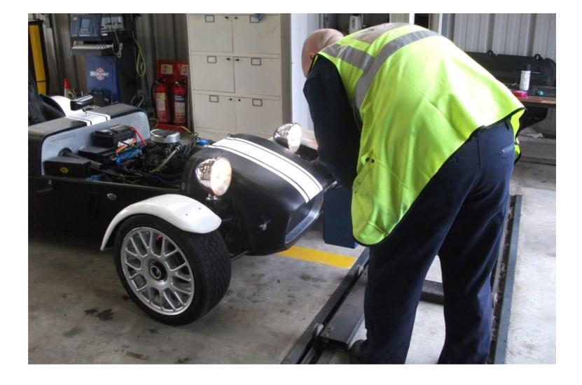
Check the headlamp aim using an approved head lamp aim tester. As part of the inspection DVSA will check for the correct:
