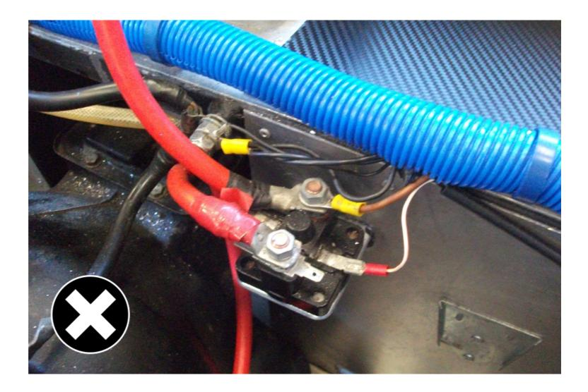
The 'solenoid' has non insulated connections with tape wrapped
