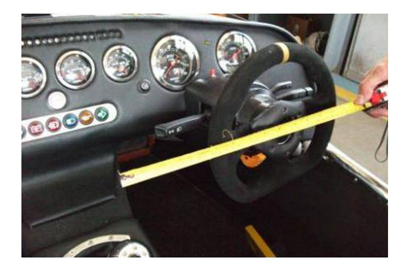
There is an exemption zone of 127 mm around the steering wheel. Anything in this zone is exempt from the inspection.
