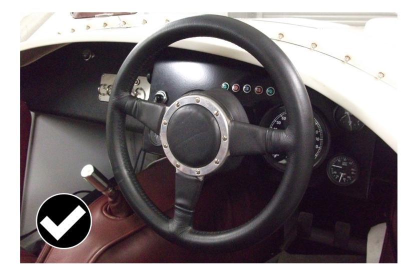
This steering wheel is nicely 'radiused', has soft protective covers on the spokes and a cushioned centre part.
