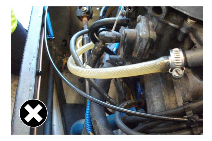
In the image above the petrol pipe is rubbing against the 'High Tension (HT) lead and isn't clipped into place. All pipes, wires and cables will
