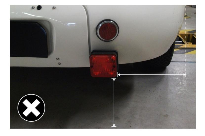
The image above shows that the fog lamp has been fitted at an incorrect height. DVSA will measure the height from the ground and the distance in from the extreme outer edge of the vehicle.
