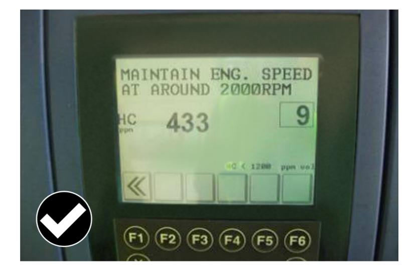
In the image above the vehicle has a pre catalyst equipped engine (this engine is from 1989). The CO is fine but the Hydrocarbons (HC) are too high.
