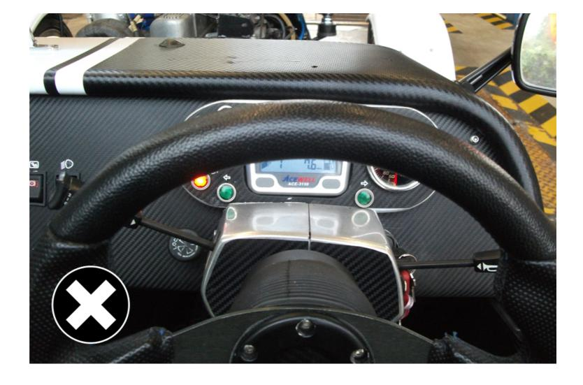
You need to be able read the speedometer at all times. In the image above the steering wheel has hidden the speedometer. This wouldn't be allowed as the driver can't see the speed they're going.
