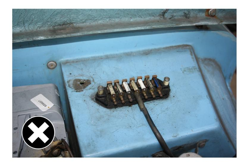
Non insulated terminals and insecure wiring aren't allowed.
