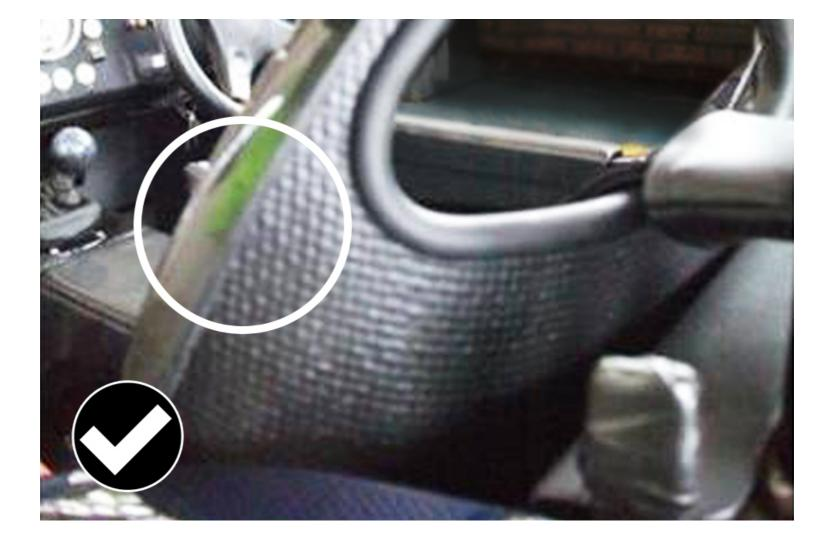
In the images above the seat edges can be contacted by the sphere and they need to be 'radiused'.
