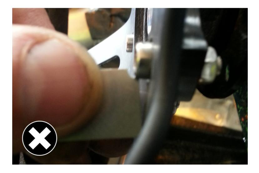
Airbags are prohibited on a non mass produced vehicle, so the steering wheel is the first thing you may hit in the event of an accident, this wheel with its 'unradiused' edges may cause injury.
