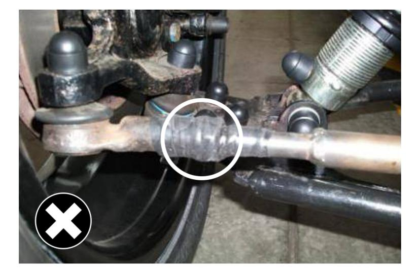
Tape wrapped around 'non radiused' edges isn't allowed. These can be easily removed and will deteriorate over time.
