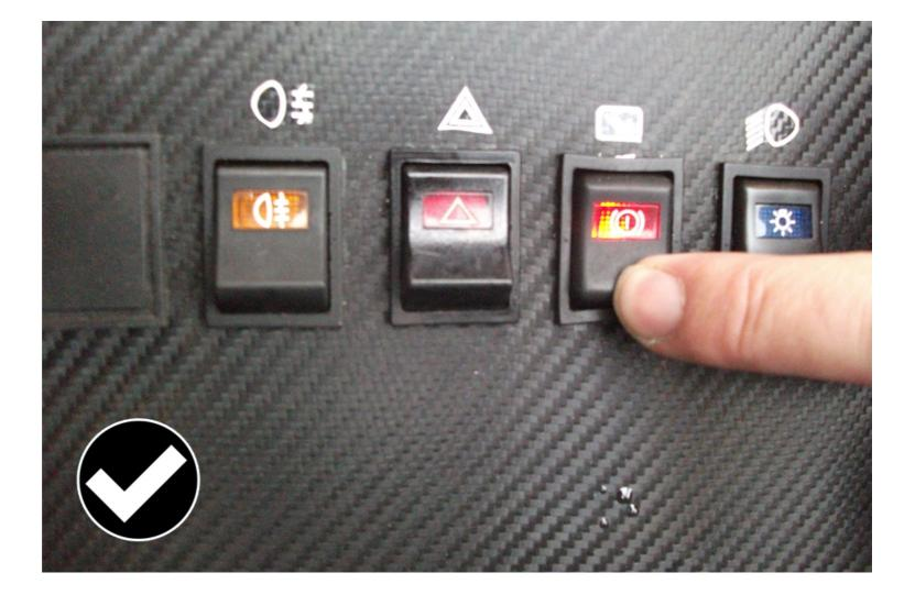
There must be a test facility to check for failure of the hydraulic braking system. This must be located within reach of the driver.
