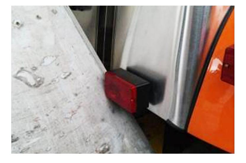
DVSA will use a 30 degree cone to determine the floor line of the vehicle. Any hard part that is an external service and is above the floor line up to 2 metres from the ground that can be contacted by the 100 mm sphere will be checked for sharp and non blunt edges.
