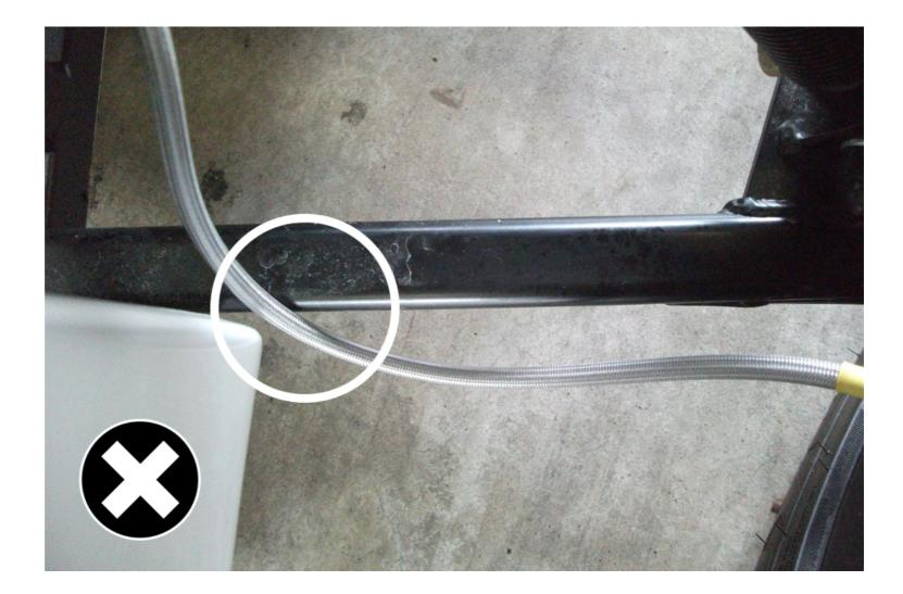
In this image the flexible brake hose is rubbing against the suspension arm. Eventually this hose would rub through and leak.
