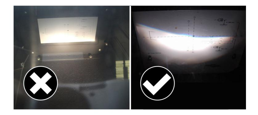
The images above show an incorrect and correct output. The headlamp aim in the incorrect example doesn't provide a clear image to allow the headlamp aim to be checked. The correct example shows
