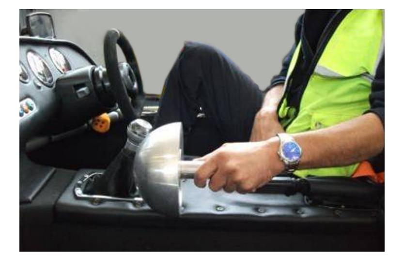
The gear lever has its own required standard. It will be checked in all forward gear positions and if contacted by sphere must be 'radiused' to 3.2 mm.
