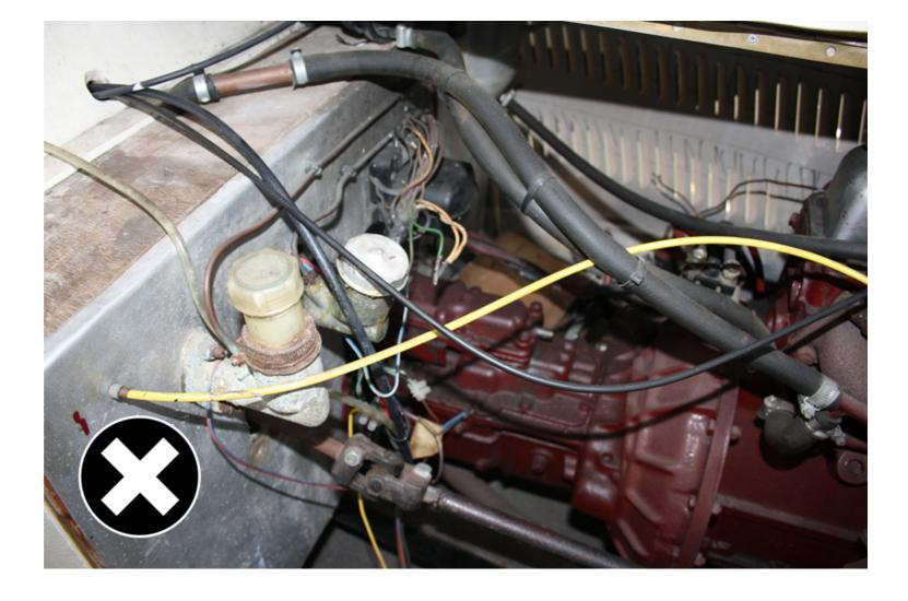
This image shows a 'brake master cylinder' that is mounted to a wooden/aluminium structure which isn't strong enough.
