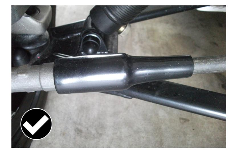
The method, in the image above, of overcoming 'non radiused' edges is allowed as it can't be easily removed and slides back to allow adjustment of the steering. These are unlikely to deteriorate.
