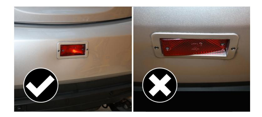
A fog lamp is a focused beam and must be fitted squarely to the rear of the vehicle.
