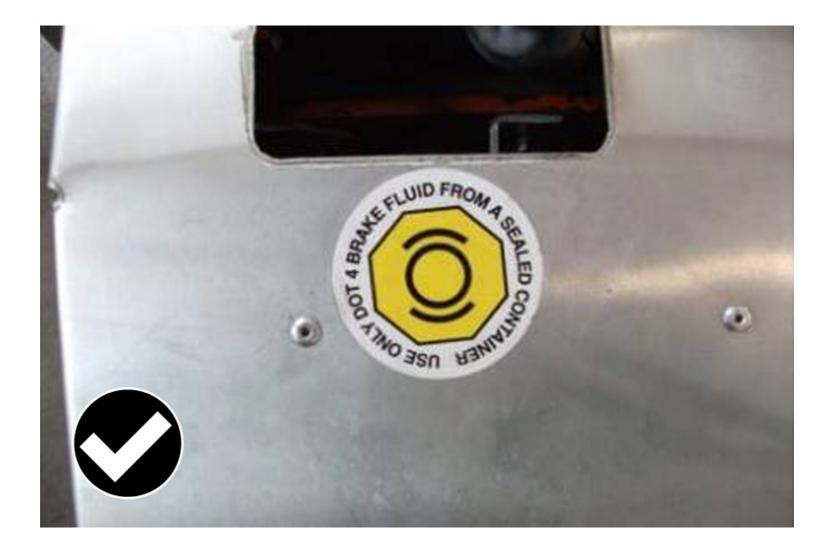
An indelible label must be fitted within 100 mm of the master cylinder that indentifies the brake fluid used.
