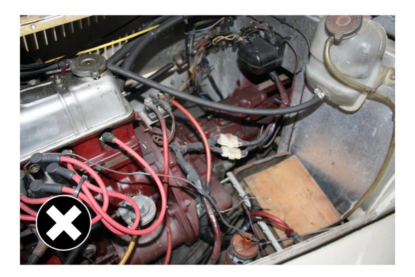
In this image there are insecure hoses, cables and wires. There are also wires that aren't insulated.
