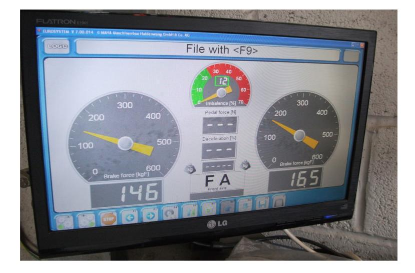
For most vehicles DVSA will carry out a full brake test on rollers to check:
