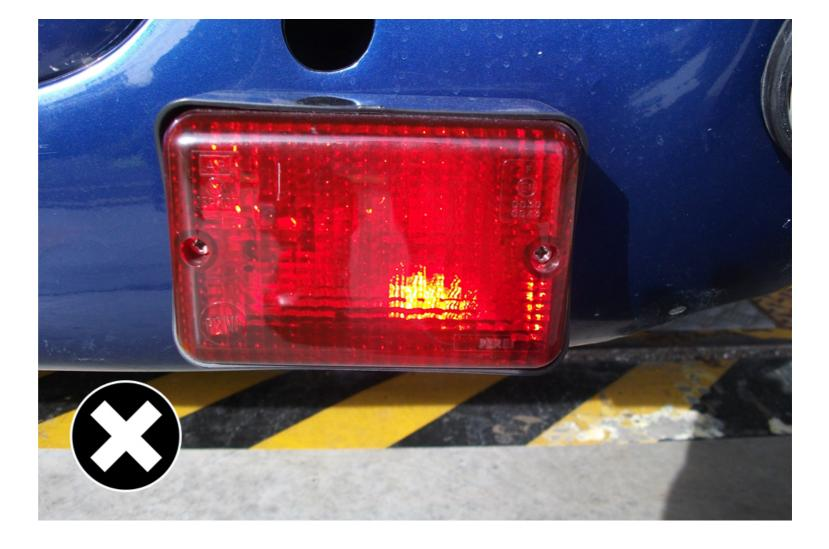
The fog lamp is correctly fitted. If it's contactable with the 100 mm sphere it may not meet the <u>required standard for exterior projections</u>.
