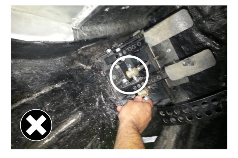
Braking ratios between axles mustn't be manually adjustable.
