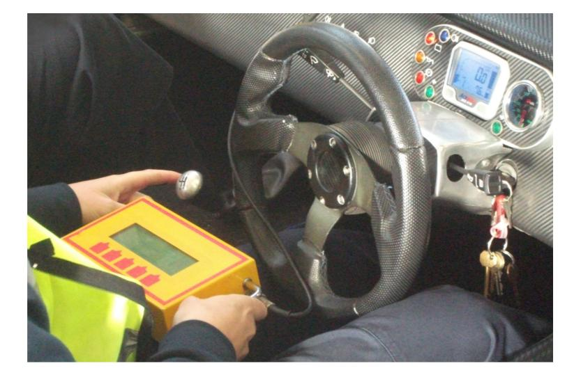
Speed will be checked for accuracy between 35 and 70 miles per hour (mph).
