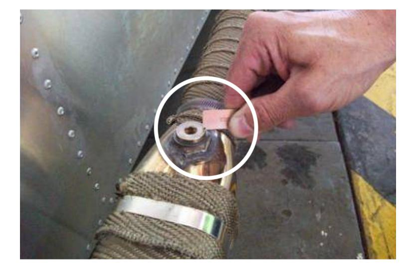
DVSA will check for items that can be contacted with a 100 mm sphere (the sphere represents your knee) and anything it touches on the exterior of the vehicle needs to be either blunted or 'radiused'.
