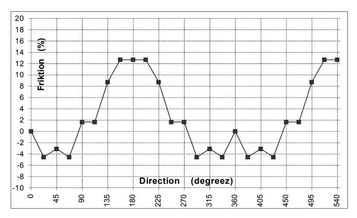
Az karnt be seen, i have massaged the friktion figurz two wayz. Firstly, the friktion with the nap (ie at 00°) iz taken az being 100% by definition. Secondly, i hav called this value 0%.
