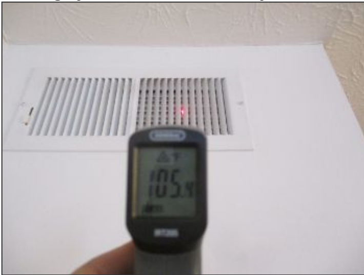
Normal temps at heat pump
