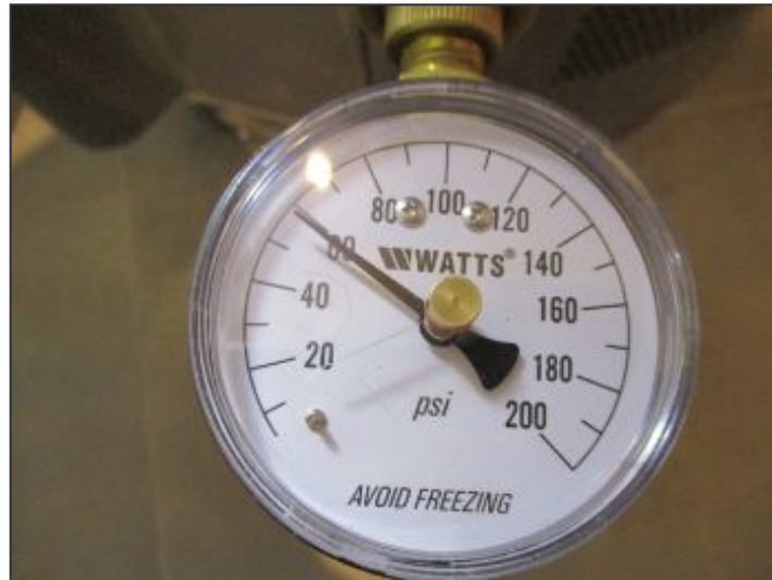
60 PSI normal at water heater
