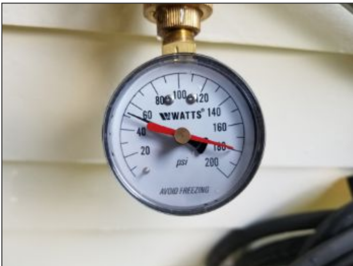
Water pressure normal at 52 PSI
