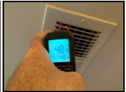
Basement level supply air temperature reading (48 degrees)
