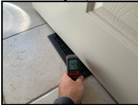
Main level supply air temperature reading (42 degrees)
