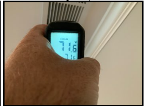
Second floor return air temperature reading (71 degrees)
