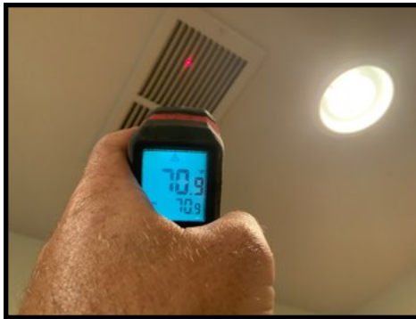
Basement level return air temperature reading (70 degrees)
