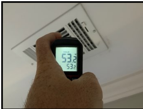
Second floor supply air temperature reading (53 degrees)
