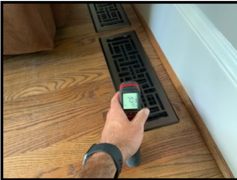
Main level return air temperature reading (70 degrees)
