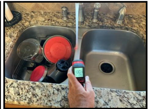
Hot water temperature reading (130 degrees)
