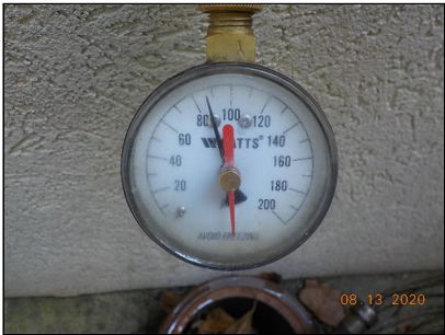
The water pressure was recorded at 88 PSI
