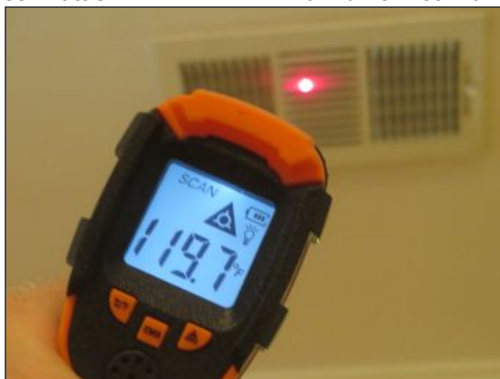
Gas furnace heating normally - 119 degrees
