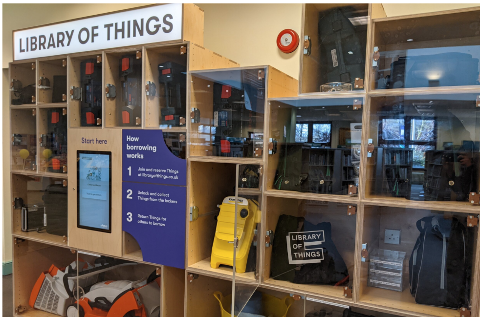
Pictured: Library of Things' self-serve item borrowing lockers installed in Morden Library. Lockers are pre-agreed standard-sizes to fit our Things. Our borrowing software pictured on the screen connects to the electronic locks via a Raspberry Pi.
