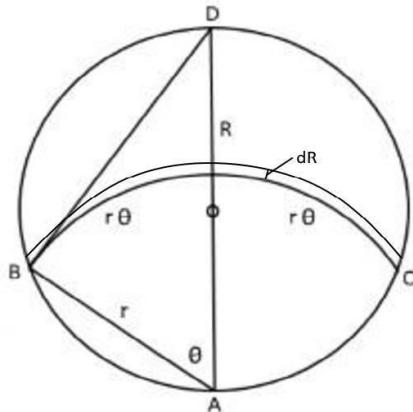
1. BC is a circular arc of radius  $r$  centered at point A. the Length,  $L$ , of BC is  $2\Theta r$ .
